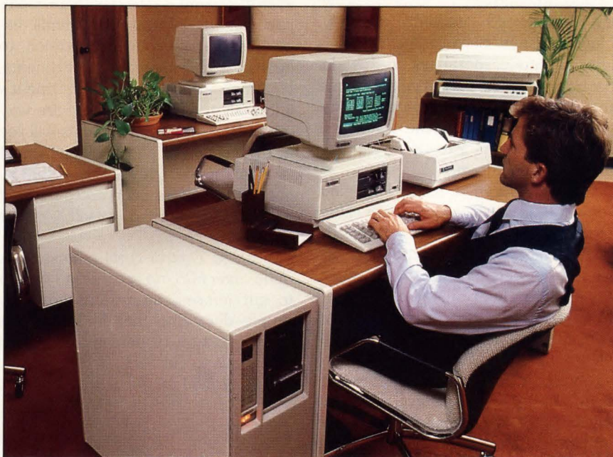
The new Harris 9300 controller (in foreground) can connect up to 16 Harris or IBM micros and/or IBM 3270-type terminals to a host with the aid of a Lanier 9178 communications link (far right).
