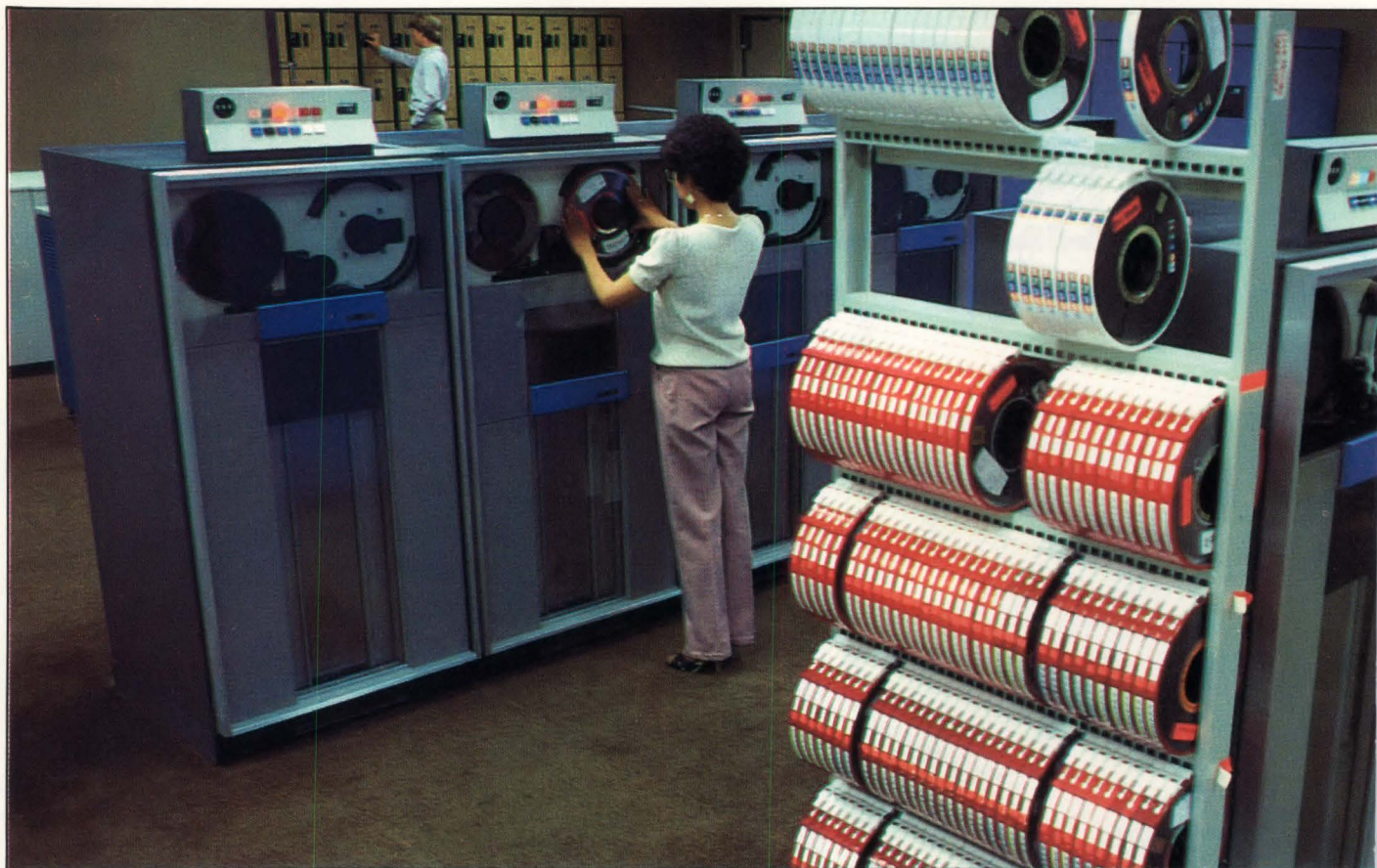
Westlake Service Center has 12 IBM 3420 tape drives, and 12 Burroughs 9495-23 and 9495-22 tape drives (above). Color-coded tapes identify stored information. Tapes, which back up data stored on disks, also provide an economical means of transferring information between computers.
