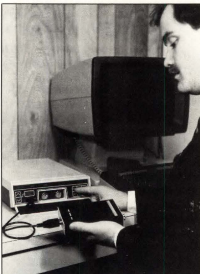
An IRE Scrambler (a data-encryption device) at a word-processing center encrypts documents as information is transmitted through a modem to a remote office.
