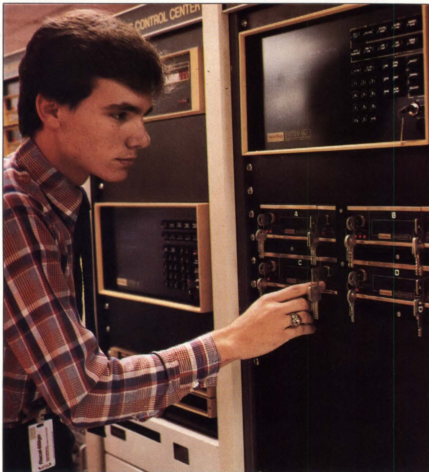
Simply by pressing a test button, an operator can easily perform routine diagnostic testing on a Racal-Milgo Datacryptor II. This unit uses the DES algorithm and is priced at $2,100.
