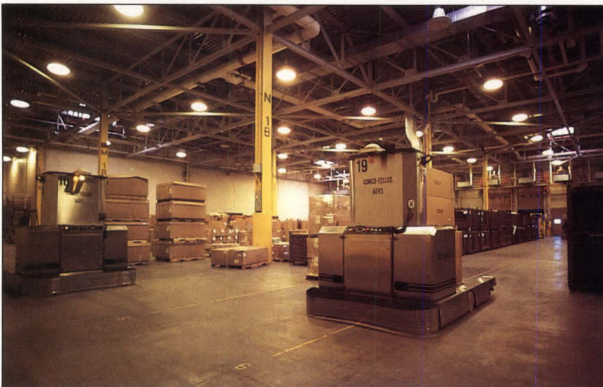
A guided vehicle—one of 22—delivers manufacturing materials from a receiving dock to the trim and chassis department at GM's Orion Township plant. A planned MAP network will integrate these vehicles with other automated resources.
