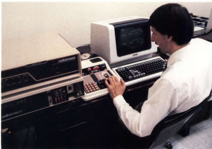
Here, an emulator is being used to test the SP/8200 and MPAC 2000 async PADs.
