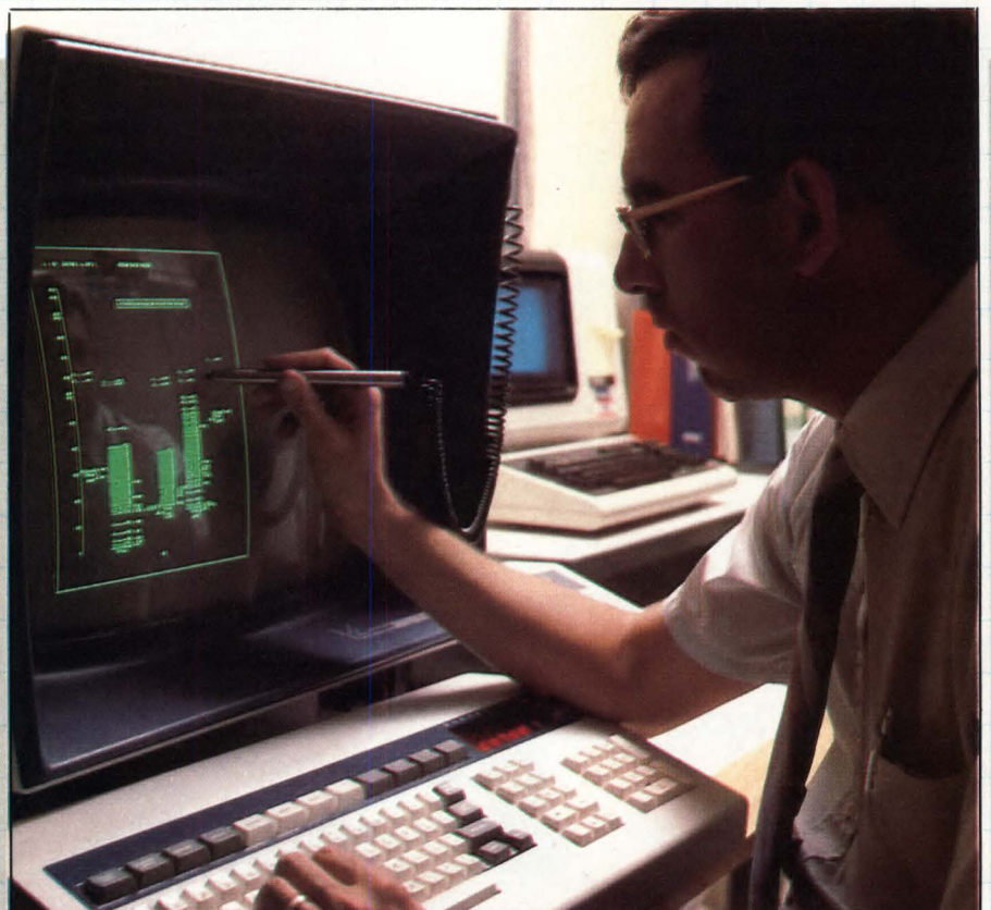
Using a light pen, Bruce Barton, computer-science analyst, draws and manipulates images on the display of Graphicus 80, an interactive graphic-display system manufactured by Vector Automation (right).
