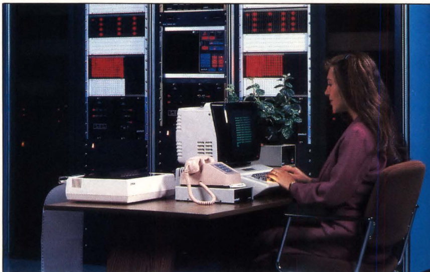
Data-over-voice (DOV) communications simplify wiring requirements to workstations by using the same twisted-pair telephone wiring for both voice and data communications. Pictured here is the Line Miser DOV (under the telephone) from Gandalf Data Inc.
