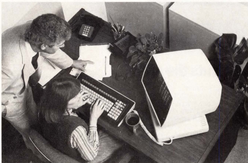
The 8000 Series intelligent terminals from Zentec Corp., Santa Clara, CA, feature ergonomic design: Each terminal swivels 60 degrees and tilts 20 degrees; the screen is glare-free and comes in white, amber, or green phosphor. Communicating in synchronous or asynchronous modes, this terminal lists for $1,750.
