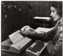
other systems or compatible terminals for: remote computing, database accessing and timesharing, interfacing with the TWX/Telex network, and printing for any crt with RS-232 interface. Price: \$750. Six to eight pages of material can be typed offline and sent from memory for efficient use of online
