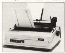
\$400. It features full form-handling capability and variable paper positioning from 7 to 14 inches. It feeds up to 200 sheets of paper by itself and attaches quickly without tools or electrical connections. Ribbons and printwheels can be changed, and envelopes or labels can be inserted manually, without removal of the sheet feeder.
