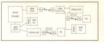
IRMA™ is the Decision Support Interface™ that gets IBM Personal Computers and IBM PC XTs into the 3270 mainstream via direct attachment to 3274 or 3276 controllers.
