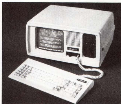
The Olivetti PC is one of several "operationally compatible" personal computers. It can run programs written specifically for the IBM Personal Computer.
