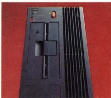
The Tower microprocessor packs a lot of computer power in a 29" x 27" x 7" package. Up to 16 operators, local or remote, can access the Tower at one time.
