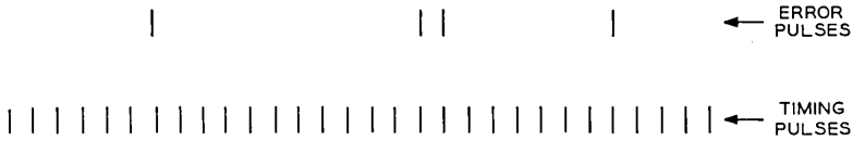
Fig. 2 — Method of error recording on magnetic tape.
