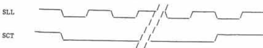
FIGURE 3.17: TYPICAL LINE AND FRAME OUTPUT SIGNALS
