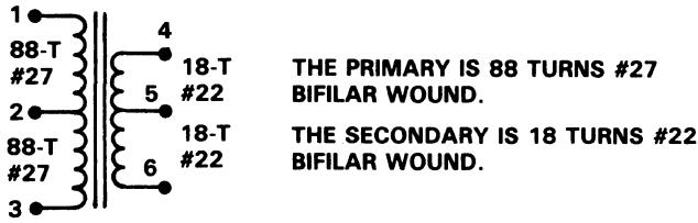
Figure 12-12. Transformer Design Data
