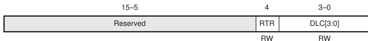
Figure 11–7. Message Control Field 0–5 (MSGCTRLn)
