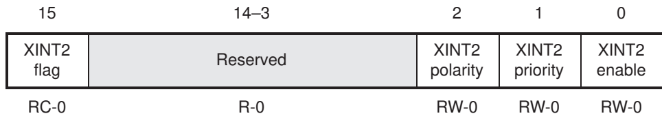
Figure 5–4. External Interrupt 2 Control Register (XINT2CR) — Address 7071h
