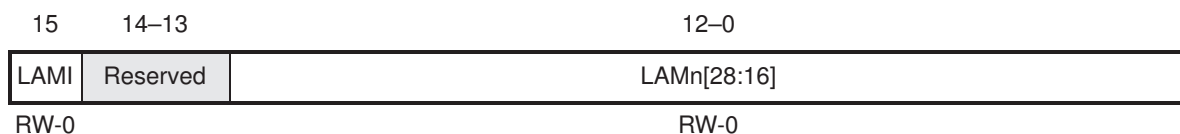
Figure 11–9. Local Acceptance Mask Register n (0, 1) High Word (LAMn_H)
