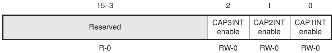
Figure 7–35. EV2 Interrupt Mask Register C — Address 742Eh
