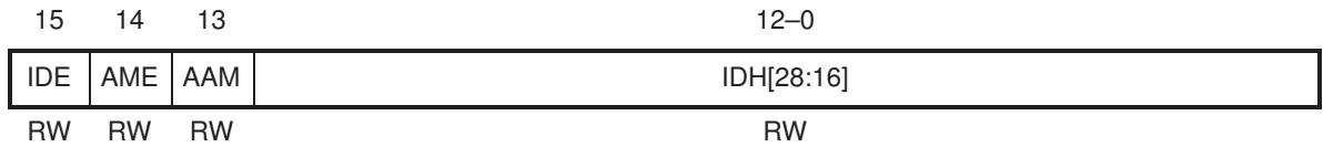
Figure 11–5. Message Identifier for High Word Mailboxes 0–5 (MSGIDnH)
