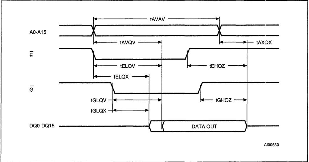
Figure 6. Read Command Waveforms
