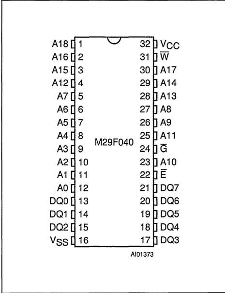
Figure 2B. LCC Pin Connections
