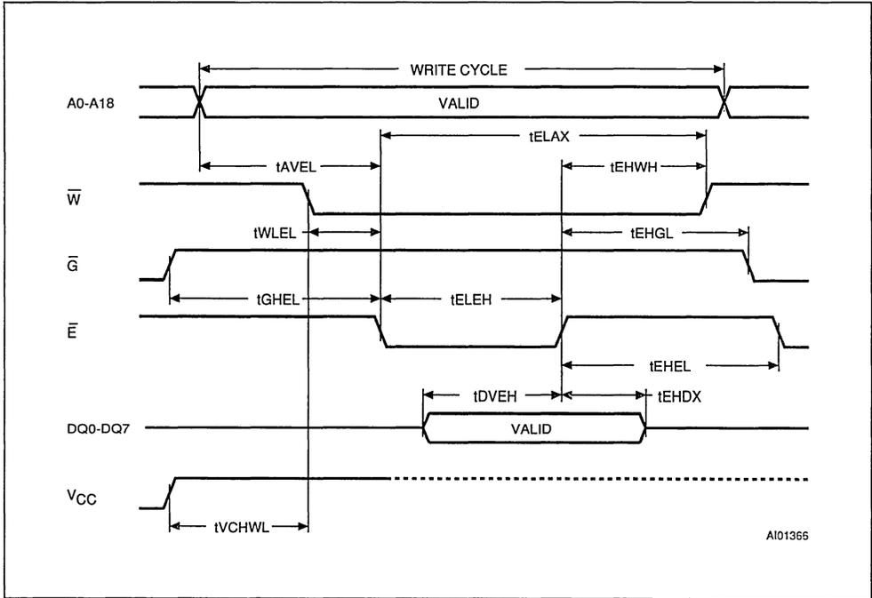
Note: Address are latched on the falling edge of  $\bar{E}$ , Data is latched on the rising edge of  $\bar{E}$ .
