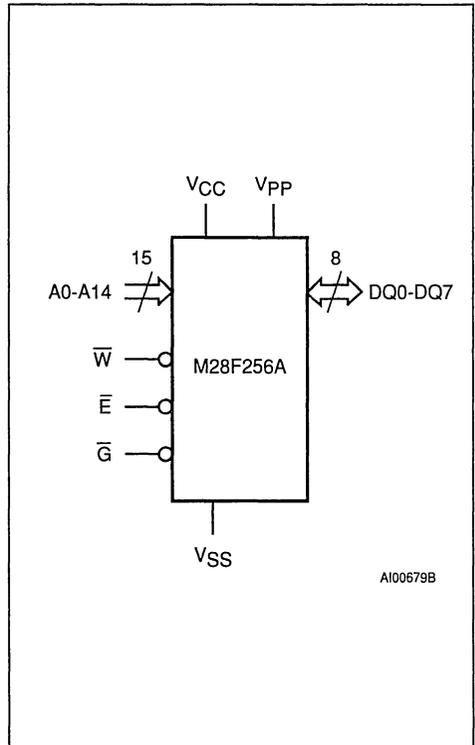
Figure 2A. DIP Pin Connections
