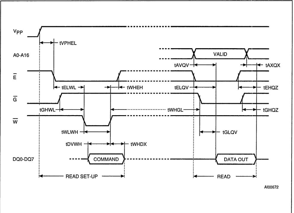
Figure 7. Electronic Signature Command Waveforms
