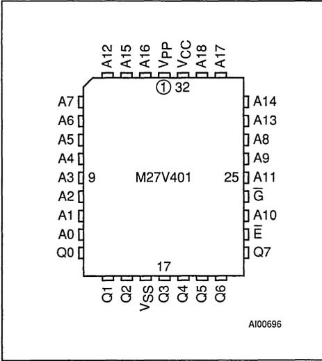
Figure 2B. TSOP Pin Connections
