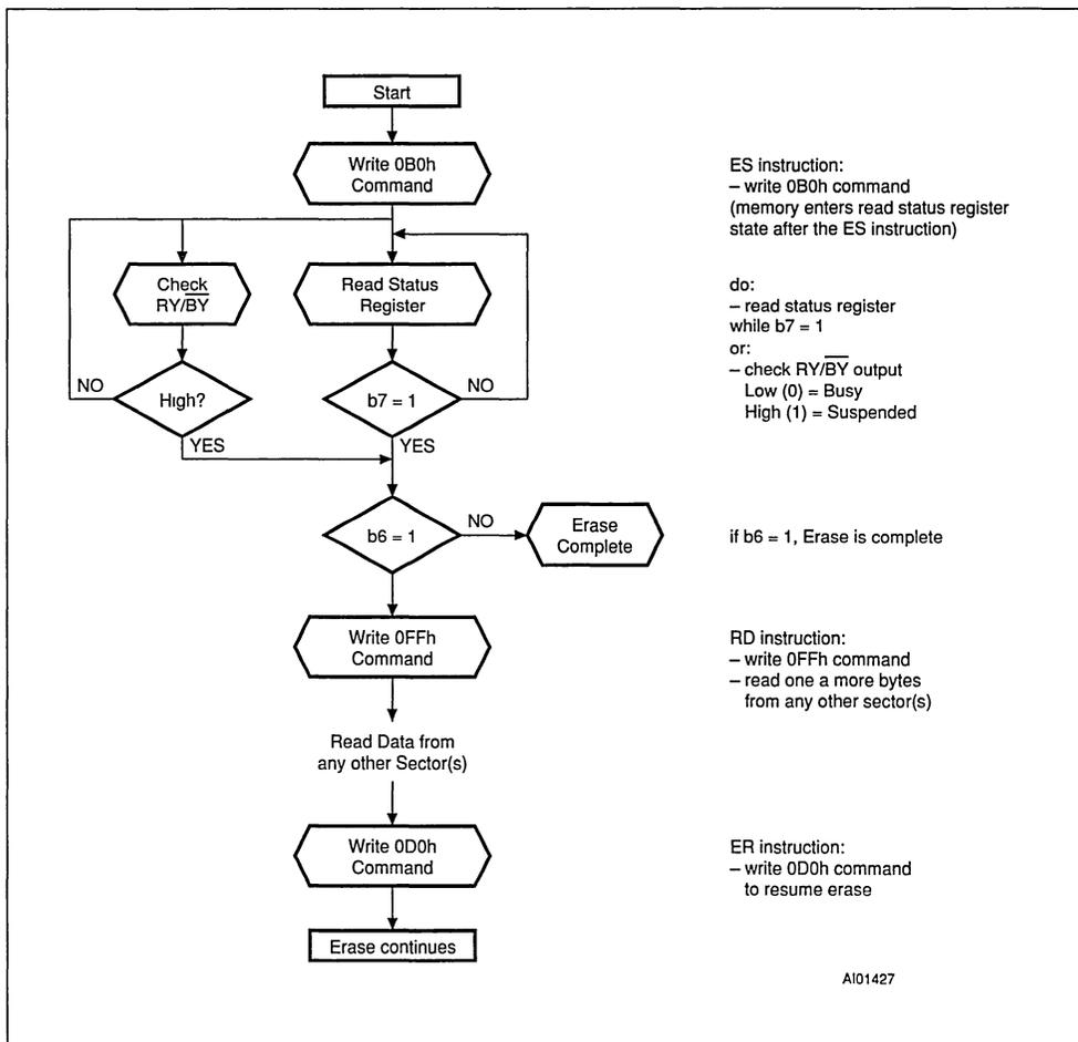
Figure 14. Command Interface and Program Erase Controller Flow-diagram (a)
