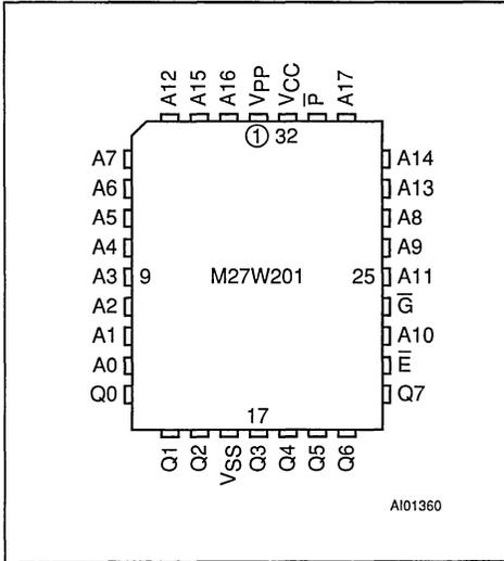
Figure 2B. TSOP Pin Connections
