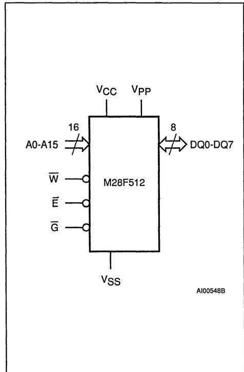
Figure 2A. DIP Pin Connections
