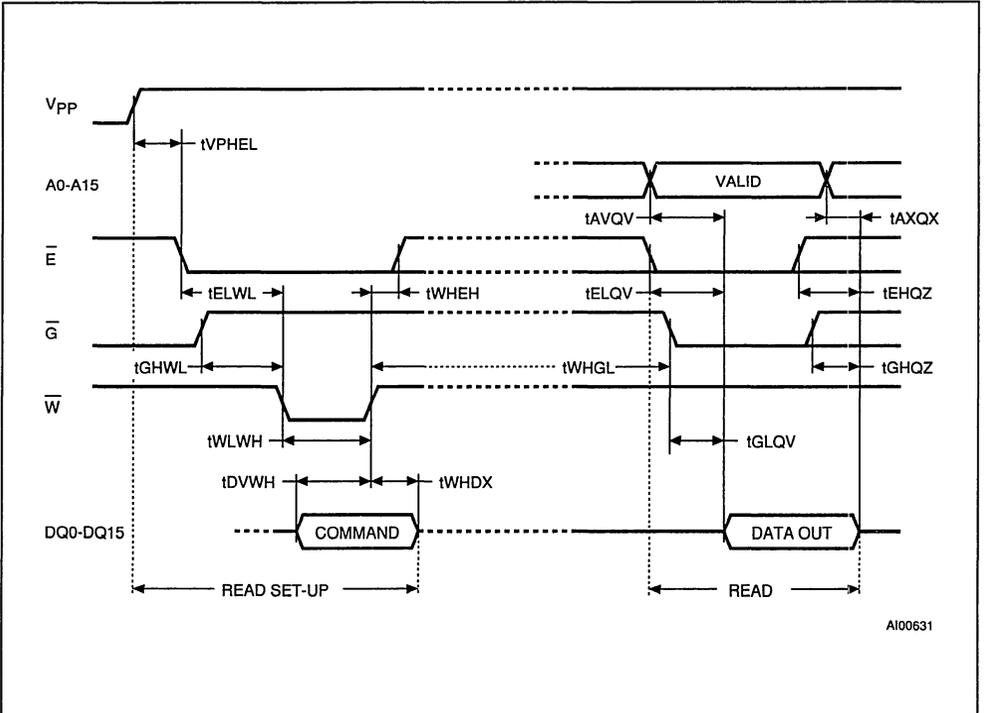
Figure 7. Electronic Signature Command Waveforms
