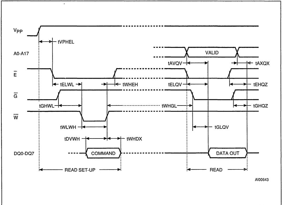
Figure 7. Electronic Signature Command Waveforms
