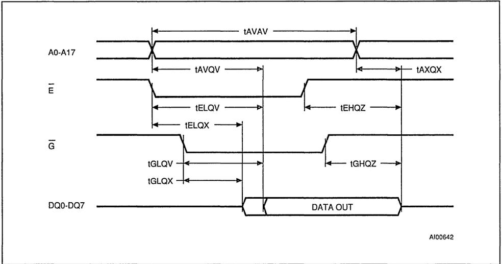
Figure 6. Read Command Waveforms
