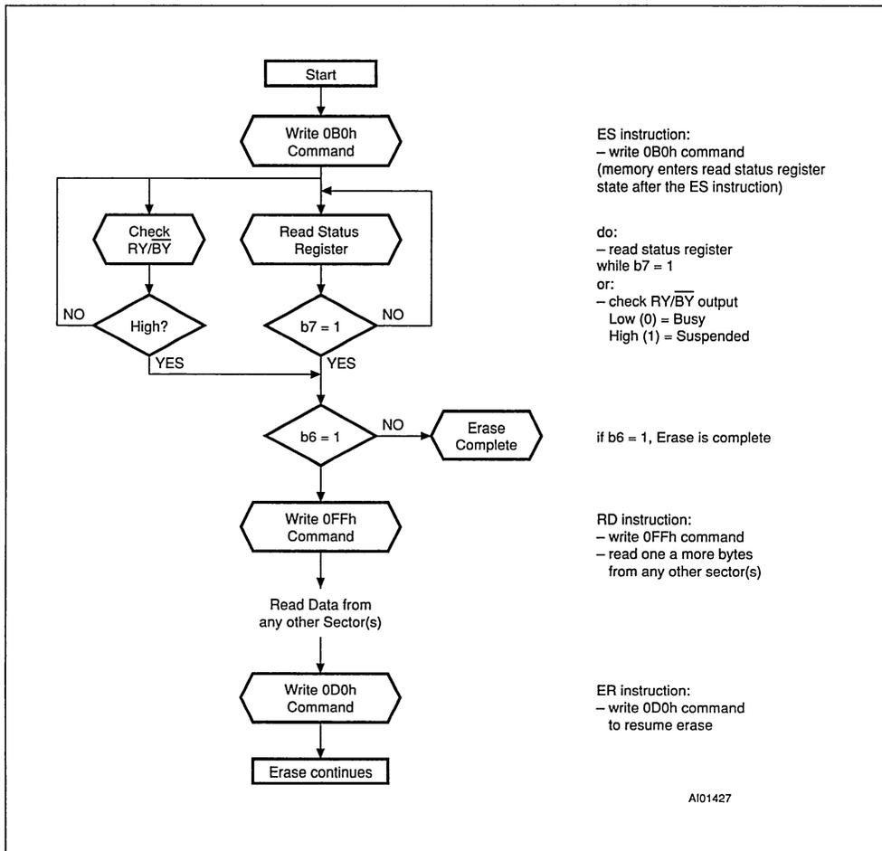
**Erase Resume (ER) instruction.** If an Erase Suspend instruction has been previously executed, the erase operation may be resumed giving the command 0D0h. The Status Register bit b6 will be cleared when erase resumes. Read operations output the Status Register after the erase is resumed.
