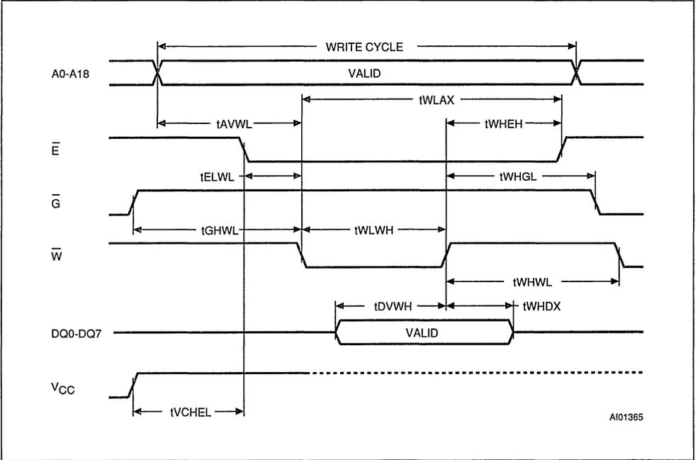
Note: Address are latched on the falling edge of  $\overline{W}$ , Data is latched on the rising edge of  $\overline{W}$ .
