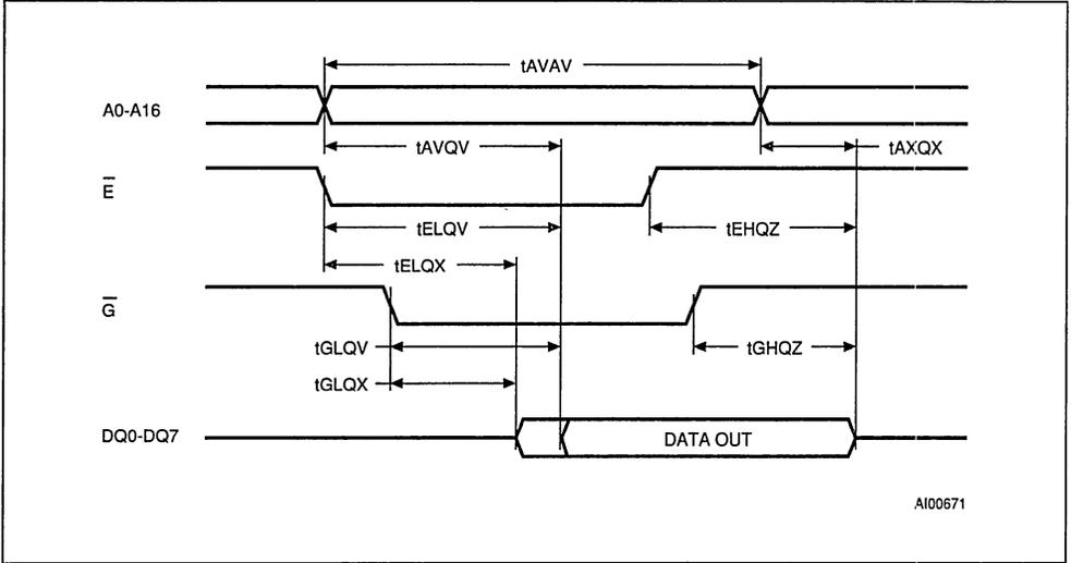
Figure 6. Read Command Waveforms
