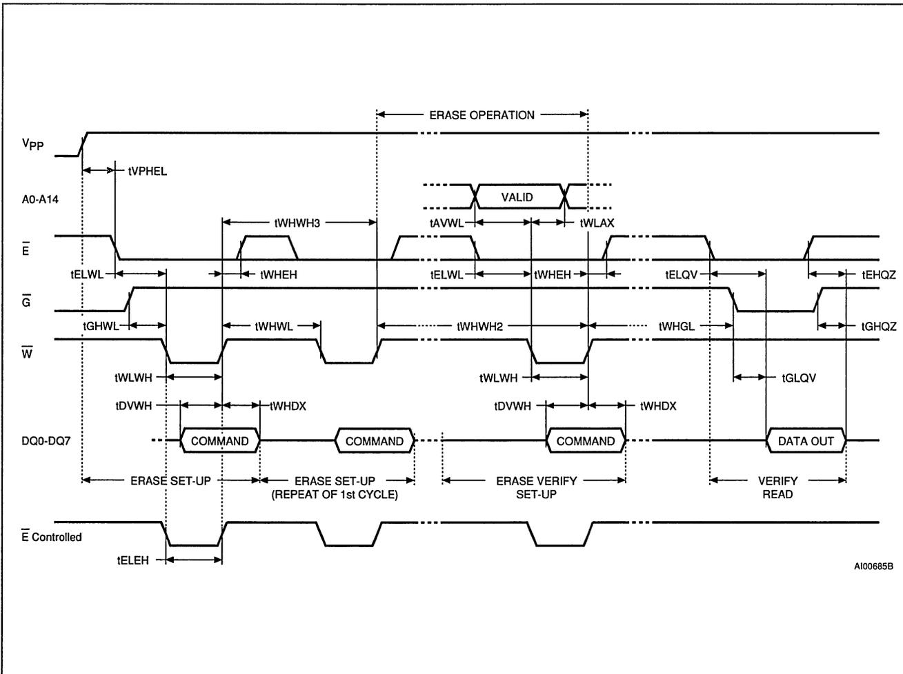
Figure 9. Program Set-up and Program Verify Commands Waveforms
