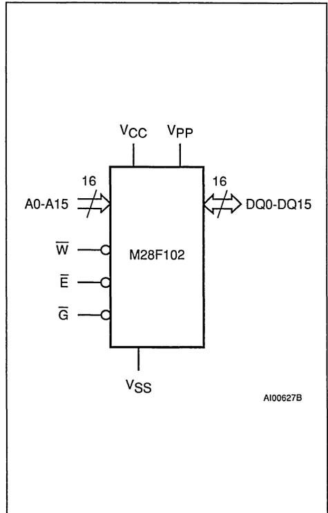
Figure 2A. LCC Pin Connections
