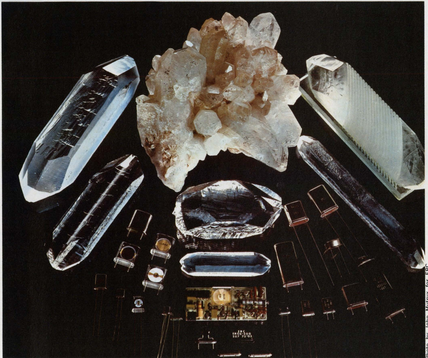
Quartz crystal wafers, sawed from synthetically grown quartz boules, are polished and mounted in a variety of packages, including glass. Electrodes are plated or de-
