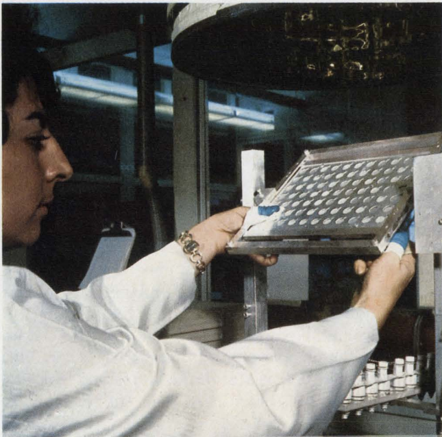
Seventy masked quartz crystals are being inserted, at Bulova Watch Co., into a fixture for vacuum deposition of electrodes. These crystals are fabricated for a TCXO.
