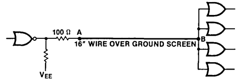
a. Wire over Ground Screen
