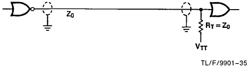
a. Single-Ended Coaxial Transmission
