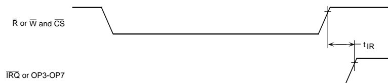
Figure A-6. Interrupt Reset Timing
