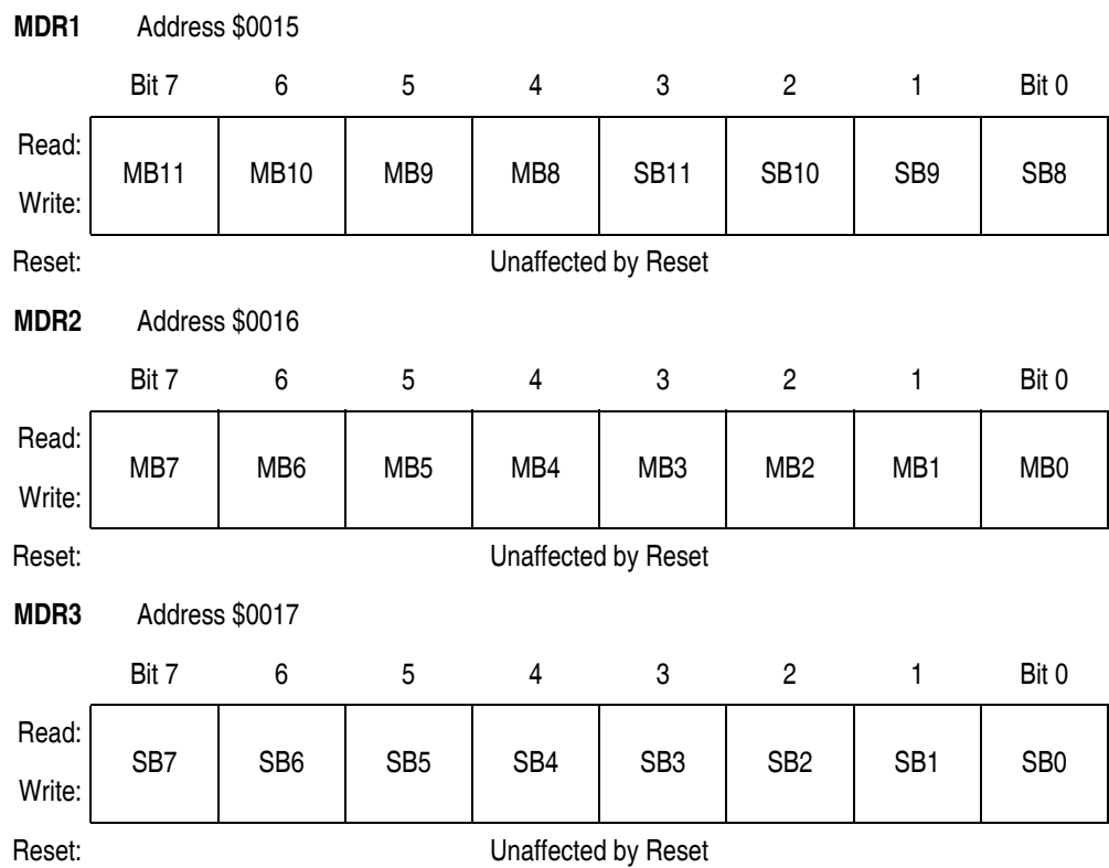
Figure 9-8. Modulator Data Registers (MDR1, MDR2, and MDR3)
