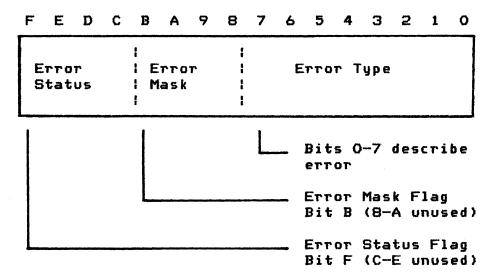
Normally, after the completion of each command, all bits of the Error Status and the Error Type are cleared (= O). The Error Mask is not affected by MDOS commands. If an error occurred during the command, the Error Status Flag (bit F) will be set by the command. In addition, an Error Type will be set into the lower half of the status word (bits O-7). The Error Type is used to indicate which error was detected by the command.
