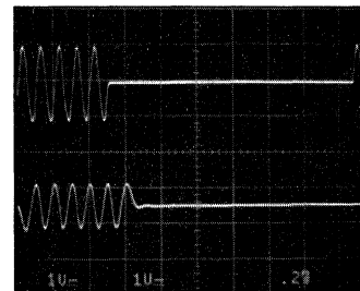
Figure 3c. Burst Response LTC1064-7, f_{CLK} = 750\text{kHz} , f_C = 10\text{kHz} , Burst: 10kHz Sine Wave
