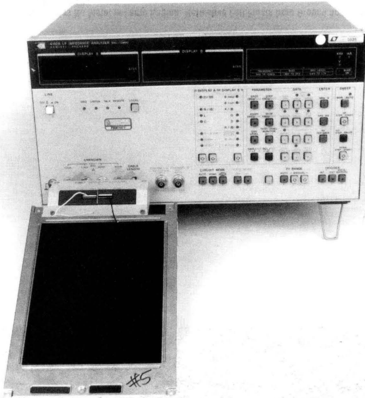
Figure 13. Measuring Lamp Wire to Display Frame Capacitance. Technique Gives Lead Wire-to-Frame Loss Information but Not Lamp-to-Foil-or-Frame Loss Data. Lamp Must Be Energized Before Its Parasitics Are Measurable
