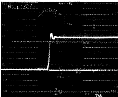
Figure C3. Expanded View of Rising Edge of LT1204 Switching from 0% to 50% (50ns Horizontal Division)
