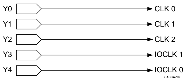
Figure 5. ispLSI and pLSI 3000 Family Global Clock Structure
