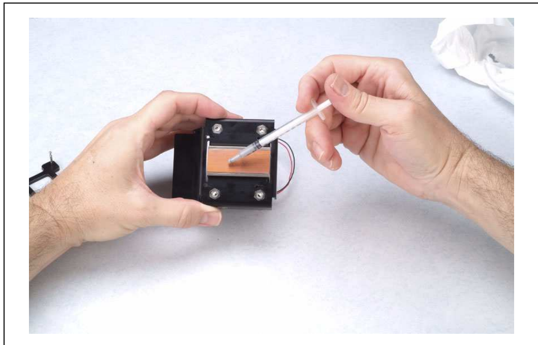
Figure 8. Applying the Thermal Grease
