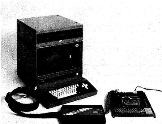
**Figure 1. A Typical 8051 Development Configuration.** The host system is an Intellec Model 225, plus 1 megabyte dual density flexible disk storage. The ICE-51 module is connected to an SDK-51 system design kit.
