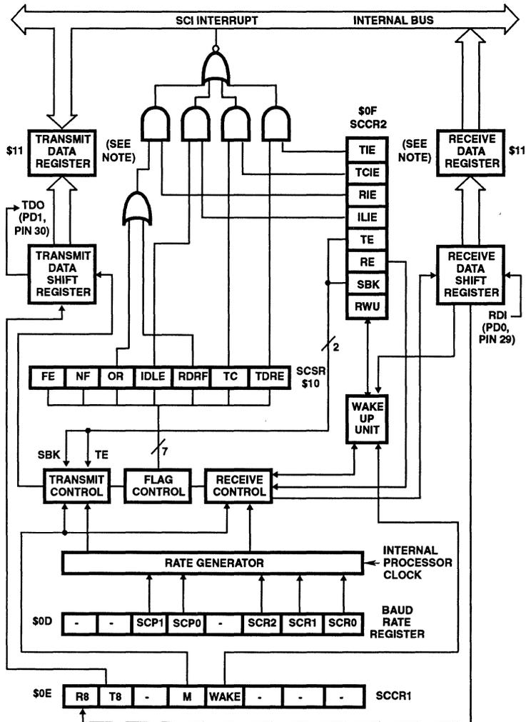
NOTE: The Serial Communications Data Register (SCDAT) is controlled by the internal R/W signal. It is the transmit data register when written and receive data register when read.
