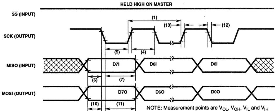
FIGURE 3D. SPI MASTER TIMING CPOL = 1, CPHA = 0
