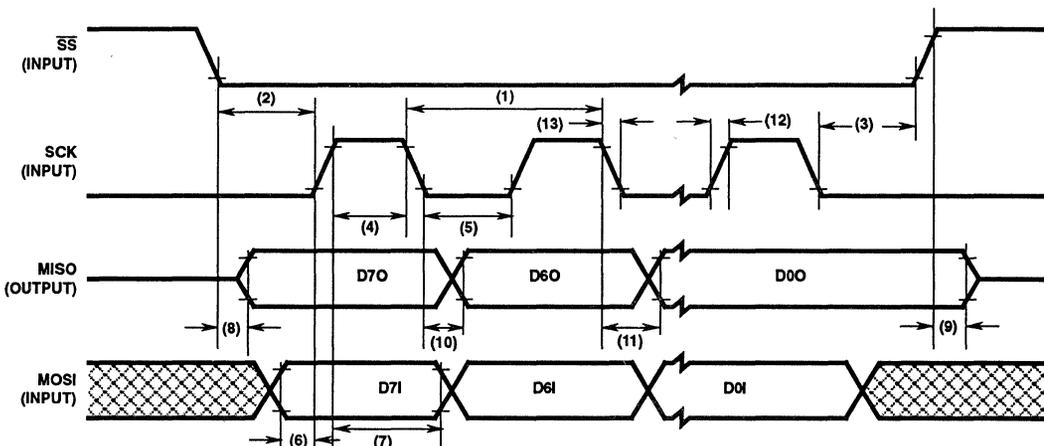
FIGURE 3G. SPI SLAVE TIMING CPOL = 0, CPHA = 0
