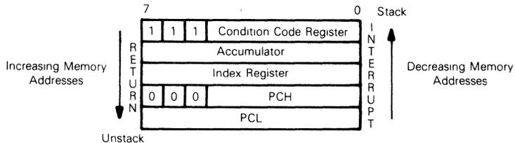
NOTE: Since the Stack Pointer decrements during pushes, the PCL is stacked first, followed by PCH, etc. Pulling from the stack is in the reverse order.
