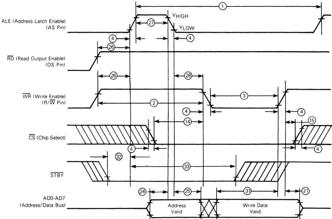
Fig. 4 - Bus write timing competitor multiplexed bus.
