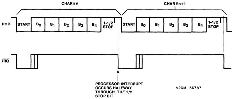
Fig. 18 - Timing with 1-1/2 stop bits.
