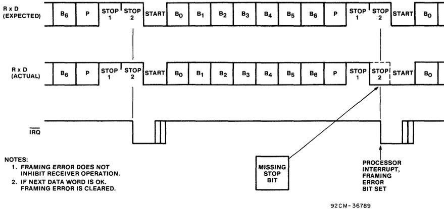
Fig. 16 - Framing error.
