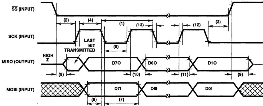
FIGURE 3E. SPI SLAVE TIMING CPOL = 0, CPHA = 1
