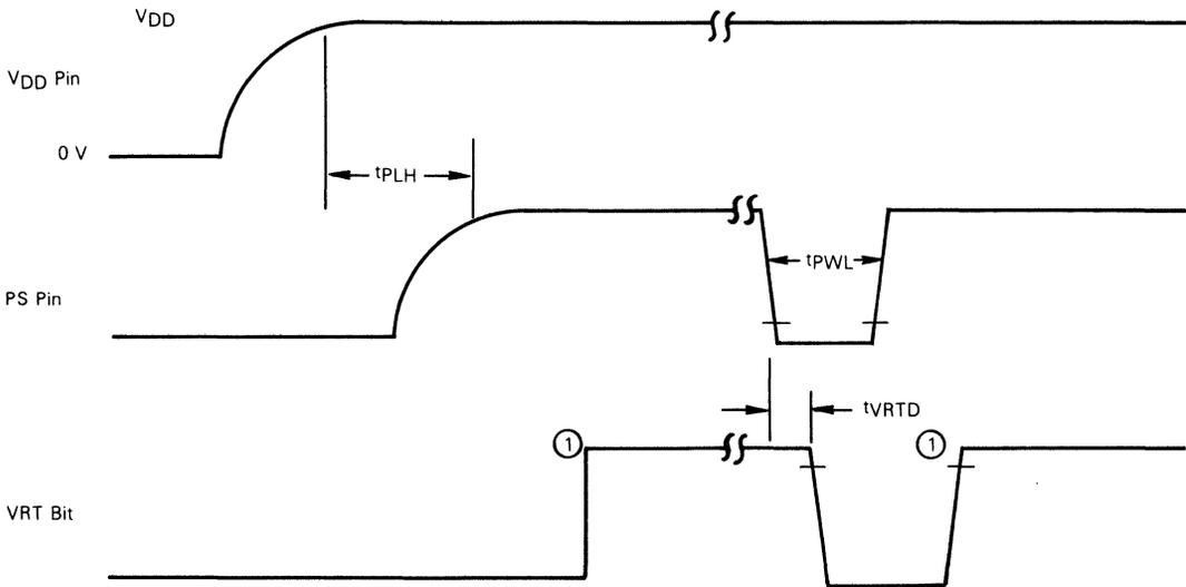
① The VRT bit is set to a "1" by reading Control Register #D. The VRT Bit can only be cleared by pulling the PS Pin low (see REGISTER D (\$OD)).
