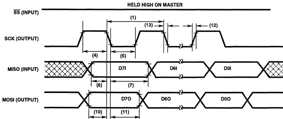
FIGURE 3A. SPI MASTER TIMING CPOL = 0, CPHA = 1
