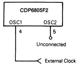
Fig. 7 - Oscillator connections.
