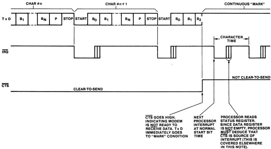
Fig. 10 - Effect of  $\overline{\text{CTS}}$  on CDP65C51 transmitter
