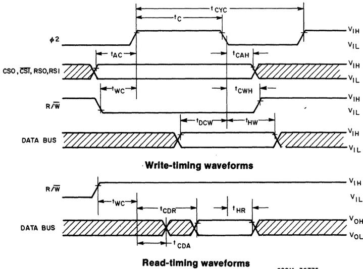
Fig. 22 - Timing waveforms.
