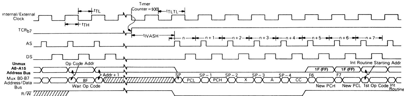
Fig. 7 – Timer interrupt after WAIT instruction timing waveforms.
