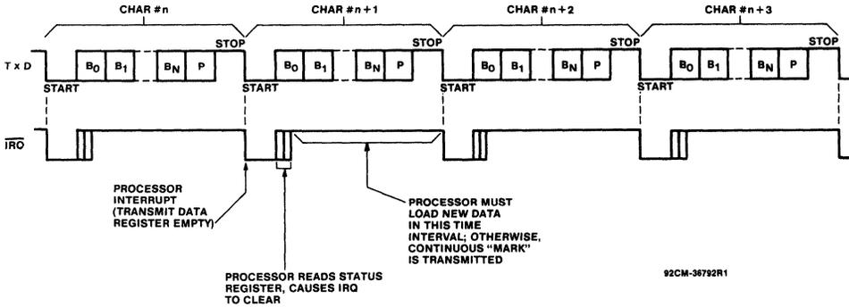
Fig. 8 - Continuous data transmit.
