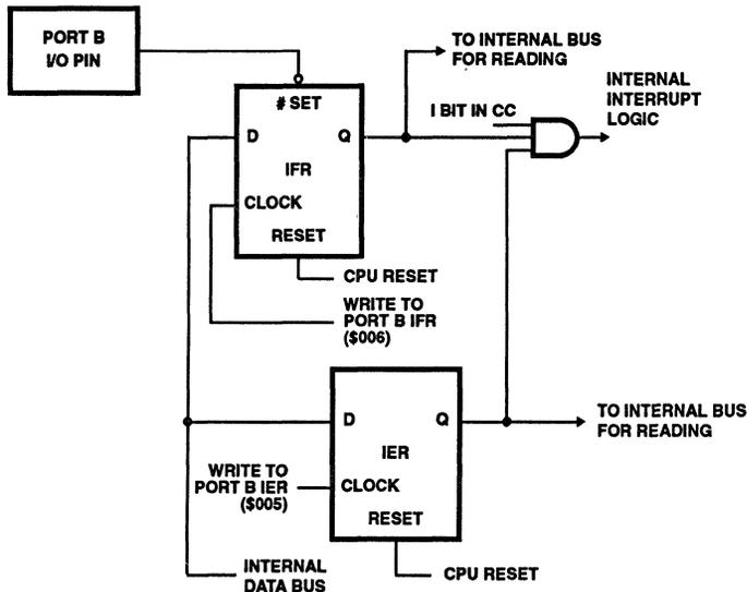
FIGURE 5. PORT B INTERRUPT LOGIC FUNCTIONAL DIAGRAM
