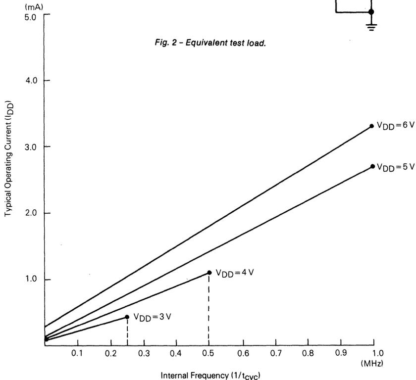
Fig. 3 - Typical operating current vs. internal frequency.
