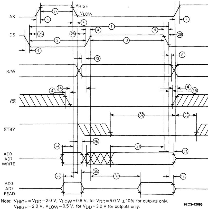
Note: V<sub>HIGH</sub> = V<sub>DD</sub> - 2.0 V, V<sub>LOW</sub> = 0.8 V, for V<sub>DD</sub> = 5.0 V ± 10% for outputs only.
