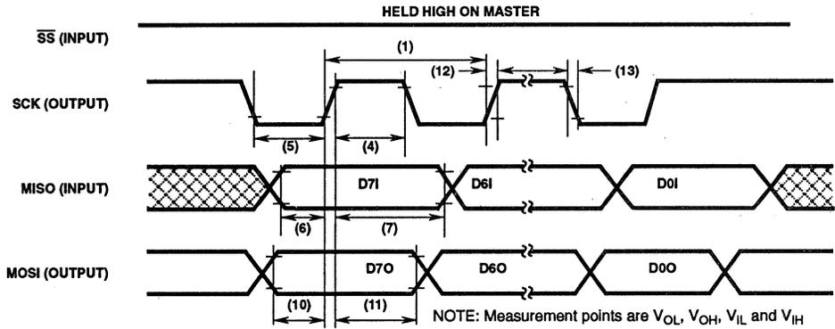
FIGURE 3B. SPI MASTER TIMING CPOL = 1, CPHA = 1
