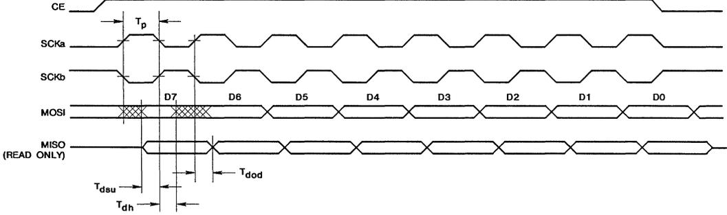
FIGURE 3. TIMING DIAGRAM FOR SERIAL PERIPHERAL INTERFACE
