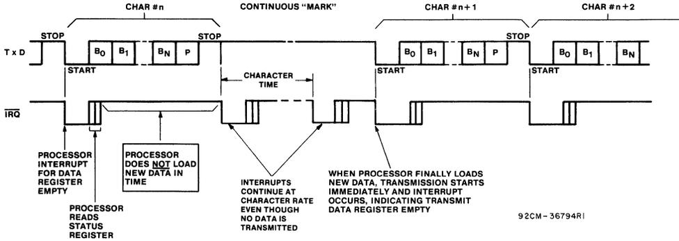
Fig. 9 - Transmit data register not loaded by processor.
