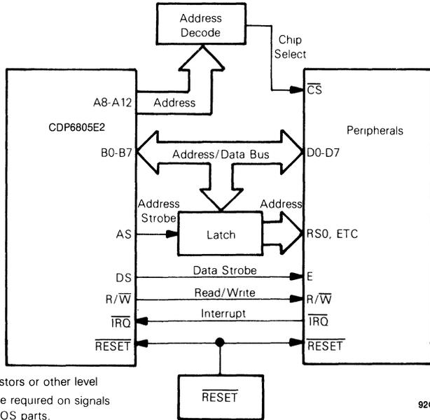
NOTE: In some cases, pullup resistors or other level shifting techniques may be required on signals going from NMOS to CMOS parts.
