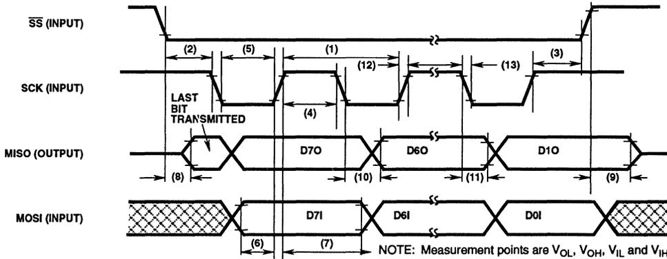
FIGURE 3F. SPI SLAVE TIMING CPOL = 1, CPHA = 1
