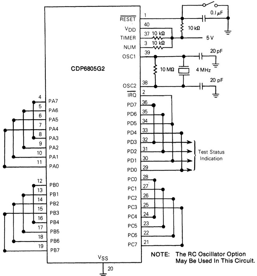
Fig. 10 - Self-check circuit.
