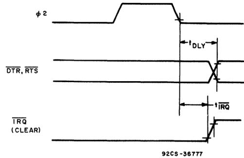
Fig. 24 - Interrupt and output timing waveforms.
