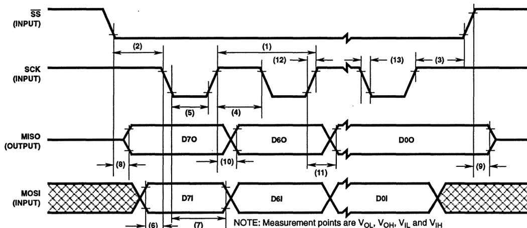
FIGURE 3H. SPI SLAVE TIMING CPOL = 1, CPHA = 0
