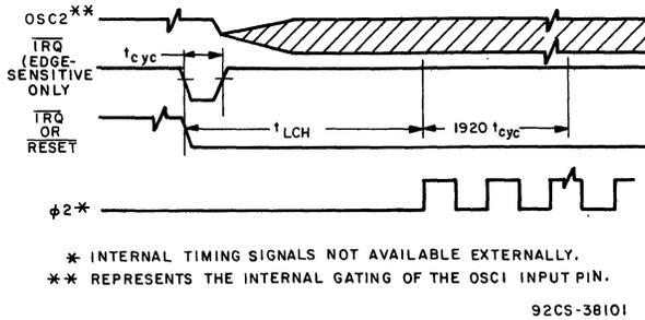
Fig. 6 - Stop recovery and power-on RESET.
