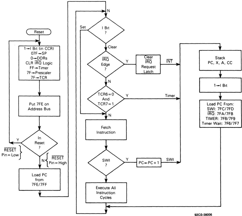
Fig. 14 - RESET and INTERRUPT processing flowchart.
