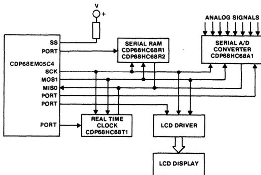
FIGURE 6. SERIAL PERIPHERAL INTERFACE (SPI) BUS SYSTEM.
