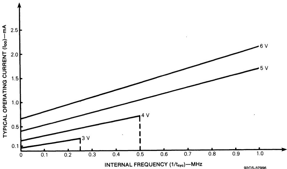
Fig. 3 - Typical operating current vs. internal frequency.
