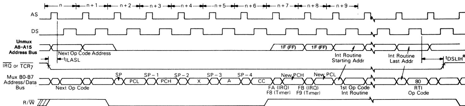
\*tDSLIIH – The interrupting device must release the IRQ line within this time to prevent subsequent recognition of the same interrupt.
