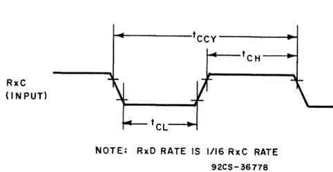
Fig. 25 - Receive external clock timing waveforms.
