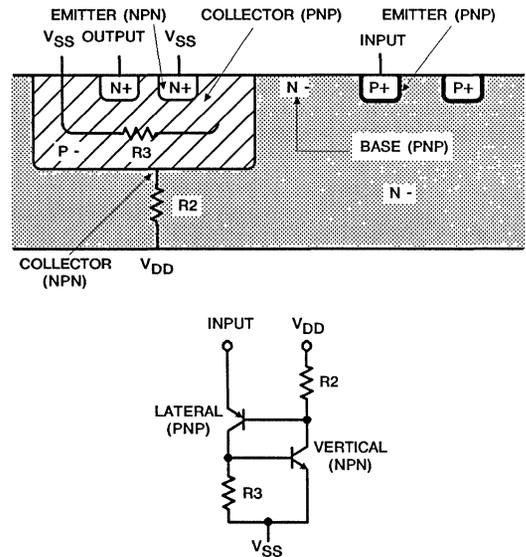
**FIGURE 5. IMPROPER BIASING CAN LATCH-UP THIS SCR CONFIGURATION.**
