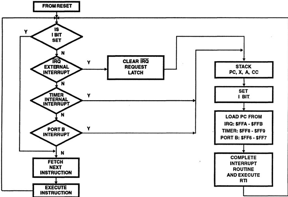
FIGURE 11. HARDWARE INTERRUPT FLOWCHART
