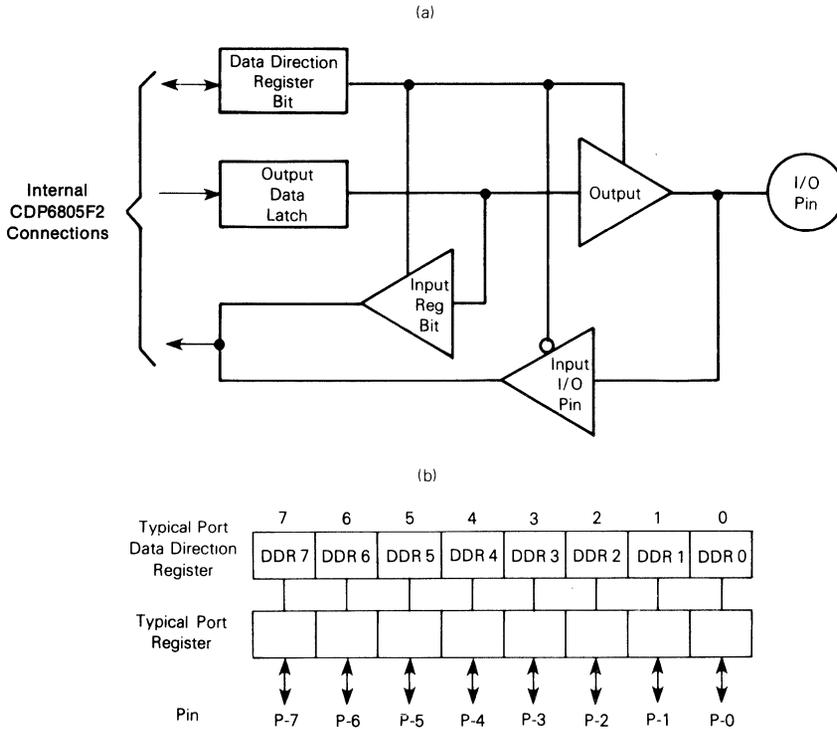
Fig. 9 - Typical I/O port circuitry.
