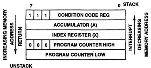
**NOTE:** Since the Stack Pointer decrements during pushes, the PCL is stacked first, followed by PCH, etc. Pulling from the stack is in the reverse order.
