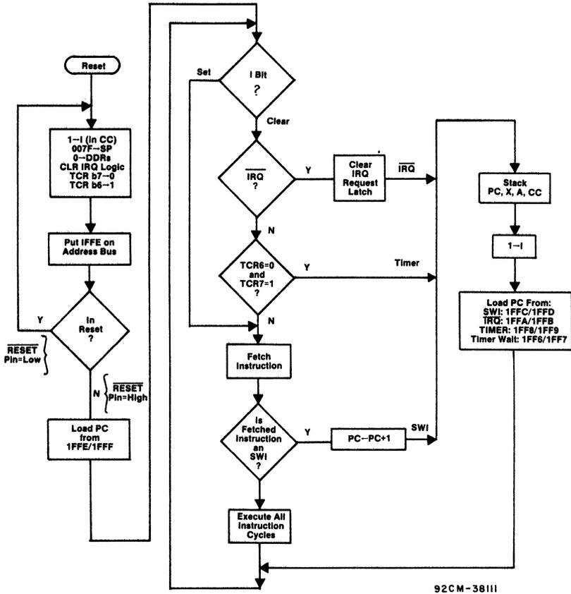
Fig. 14 - RESET and INTERRUPT processing flowchart.
