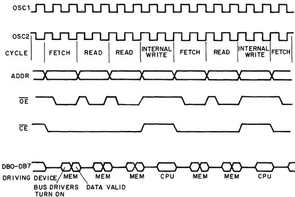
**FIGURE 2. TYPICAL CYCLE TIMING FOR THE CDP68EM05C4 EMULATOR.**
