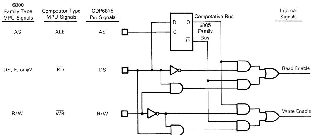
Fig. 9 — Functional diagram of MOTEL circuit.
