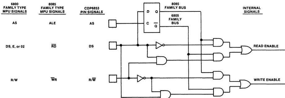
Fig. 2 - Functional diagram of MOTEL circuit.
