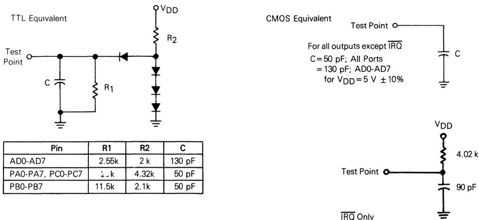
Fig. 2 - Equivalent test loads.
