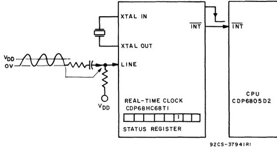
Fig. 3 - Power-sensing functional diagram.
