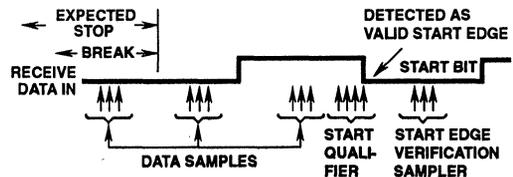
FIGURE 24. SCI START BIT FOLLOWING A BREAK
