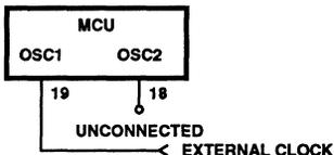
FIGURE 3F. EXTERNAL CLOCK SOURCE CONNECTIONS
