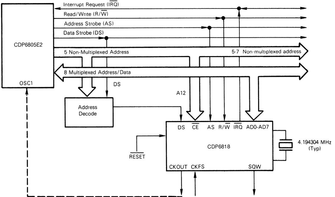
This illustrates the use of CMOS gating for address decoding.
