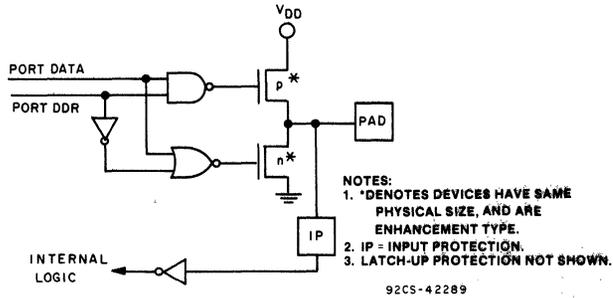
Fig. 3 - Typical Parallel Port I/O Circuitry
