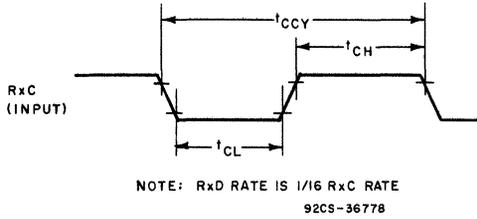
Fig. 28 - Receive external clock timing waveforms.
