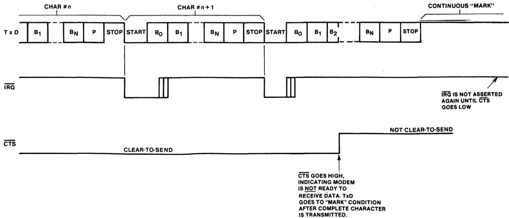
Fig. 10A - Effect of  $\overline{\text{CTS}}$  on CDP65C51A transmitter
