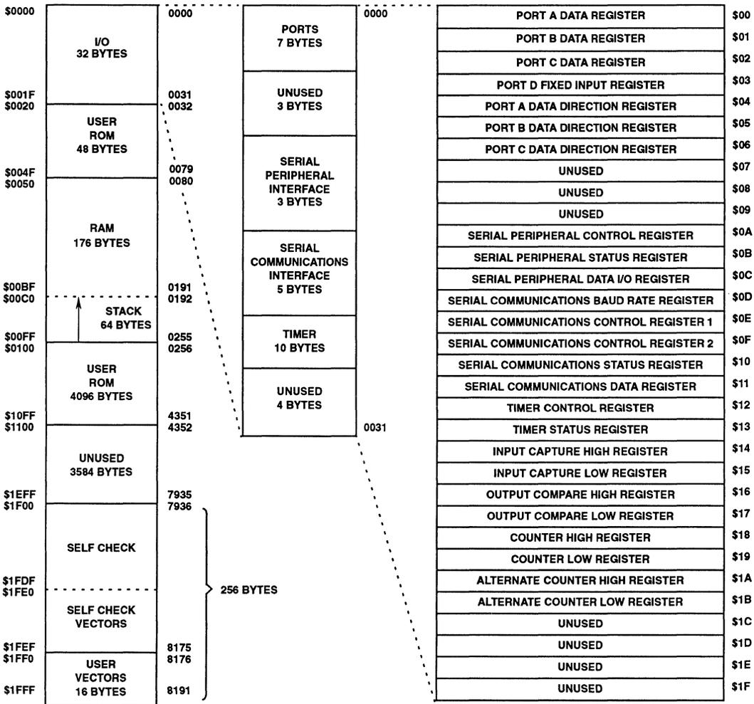
FIGURE 6. ADDRESS MAP FOR CDP68HC05C4, CDP68HCL05C4 AND CDP68HSC05C4
