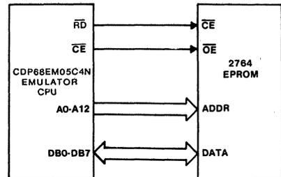
FIGURE 7. CDP68EM05C4N EMULATOR INTERFACED WITH 2764 EPROM.
