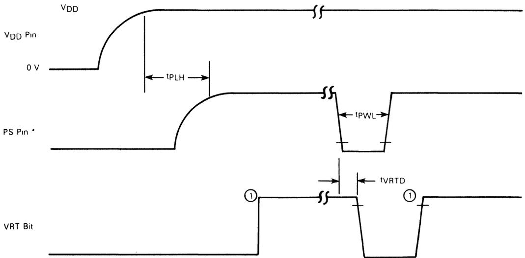
① The VRT bit is set to a "1" by reading Register d. The VRT bit can only be cleared by pulling the PS pin low (see REGISTER D (\$0D)).
