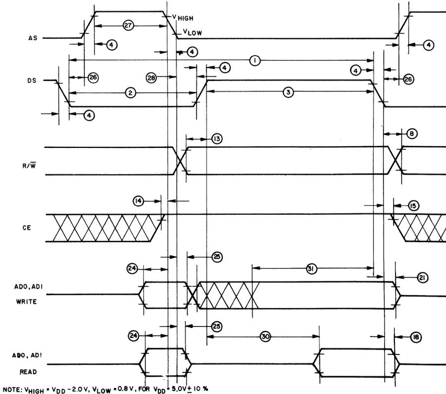
Fig. 23 - Bus timing waveforms of CDP6853.
