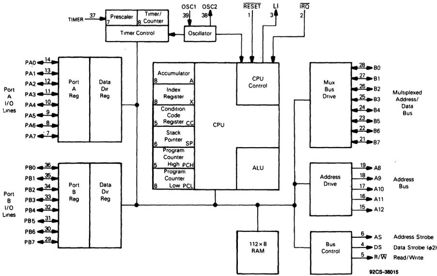
**Fig. 1a - CDP6805E2 block diagram.**
