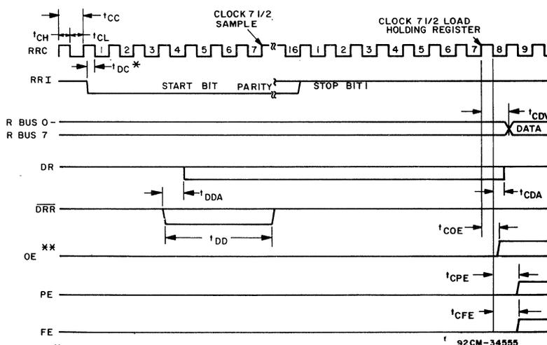
\* IF A START BIT OCCURS AT A TIME LESS THAN  $t_{DC}$  BEFORE A HIGH-TO-LOW TRANSITION OF THE CLOCK, THE START BIT MAY NOT BE RECOGNIZED UNTIL THE NEXT HIGH-TO-LOW TRANSITION OF THE CLOCK. THE START BIT MAY BE COMPLETELY ASYNCHRONOUS WITH THE CLOCK.
