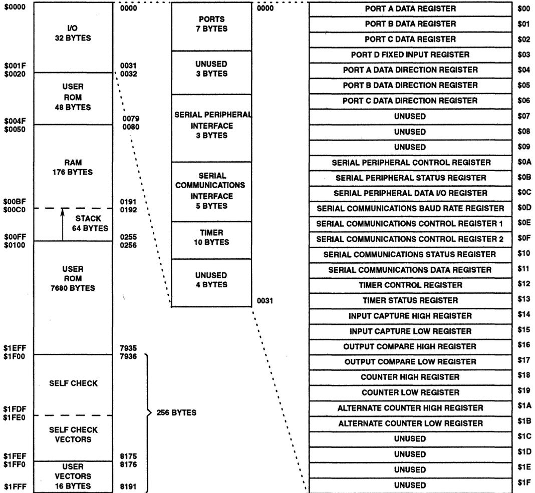
**FIGURE 7. ADDRESS MAP FOR CDP68HC05C8, CDP68HCL05C8 AND CDP68HSC05C8**
