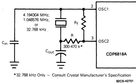
Fig. 10 - Crystal oscillator connection.
