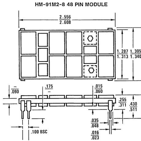
NOTE: All Dimensions are  $\frac{\text{Min}}{\text{Max}}$ , Dimensions are in inches.
