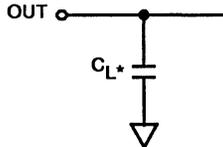
\* Includes stray and jig capacitance,  $C_L = 50pF$
