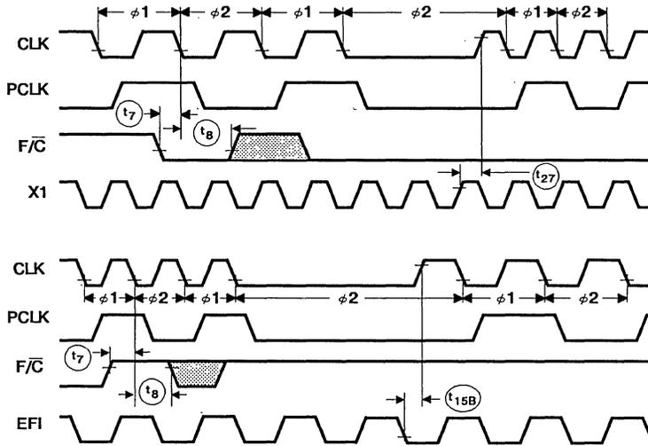
NOTE: This is an asynchronous input. The setup and hold times are required to guarantee the response shown.
