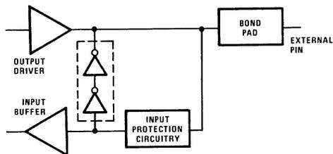
FIGURE 4A. BUS HOLD CIRCUITRY PIN 2-16, 34-39
