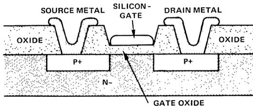
FIGURE 3. SILICON-GATE PFET STRUCTURE
