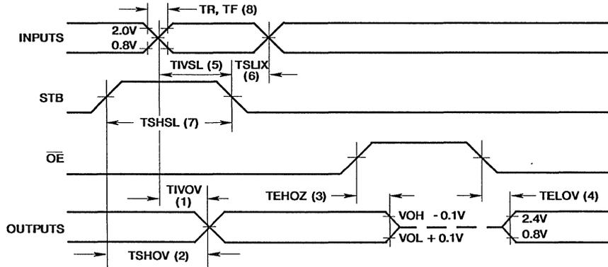
All timing measurements are made at 1.5V unless otherwise noted.
