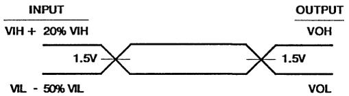
A.C. Testing: All input signals (other than CLK) must switch between  $V_{ILmax} - 50\% V_{IL}$  and  $V_{IHmin} + 20\% V_{IH}$ . CLK must switch between 0.4V and  $V_{CC} - 0.4$ . Input rise and fall times are driven at 1ns/V.
