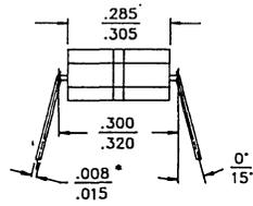
• INCREASE MAX LIMIT BY .003 INCHES MEASURED AT CENTER OF FLAT FOR SOLDER FINISH
