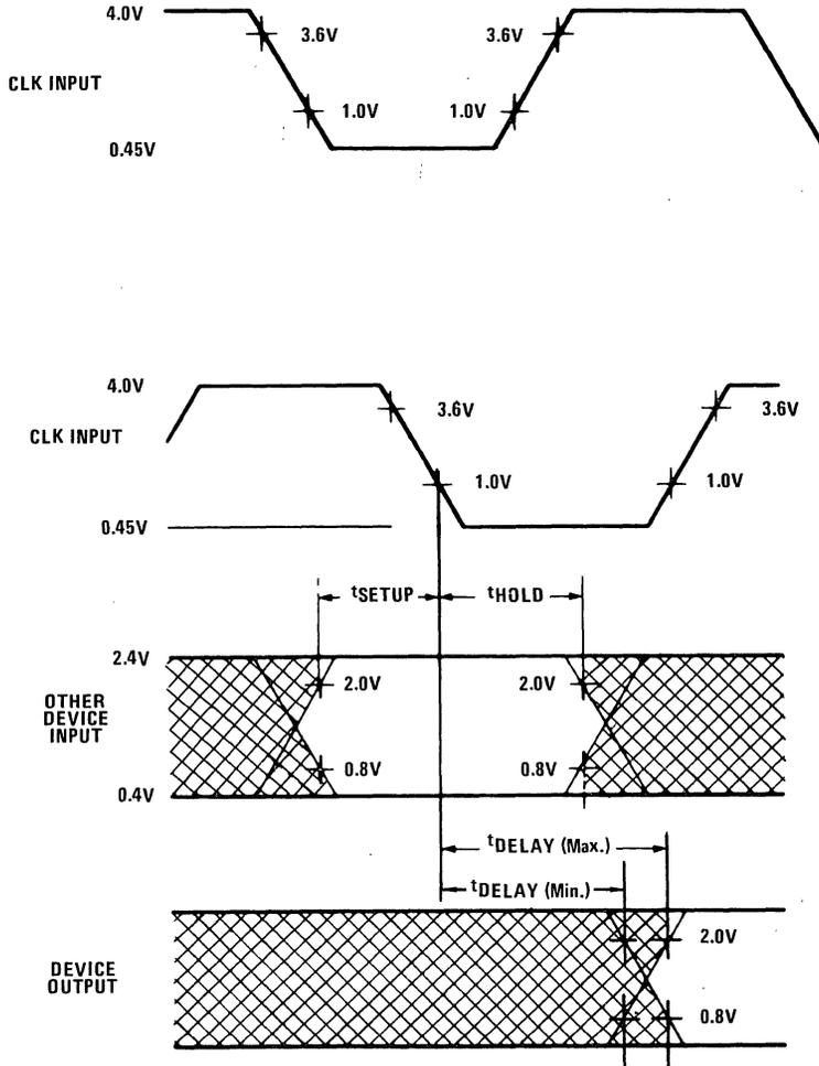
NOTE: For A.C. testing, input rise and fall times are driven at 1ns per volt.
