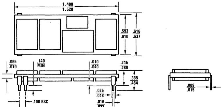
NOTE: All Dimensions are  $\frac{\text{Min}}{\text{Max}}$ , Dimensions are in inches.
