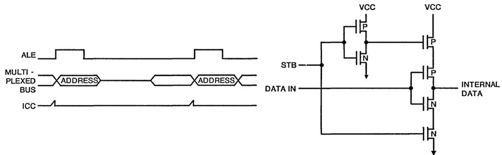
FIGURE 3. SYSTEM EFFECTS OF GATED INPUTS
