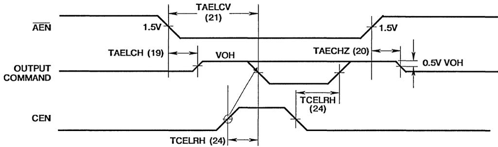
NOTE: CEN must be low or invalid prior to T2 to prevent the command from being generated.
