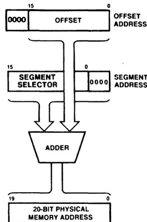
**FIGURE 7. 80C286 REAL ADDRESS MODE ADDRESS CALCULATION**
