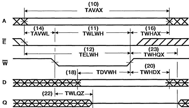
WRITE CYCLE II:  $\overline{E}$  CONTROLLED (Note 2)
