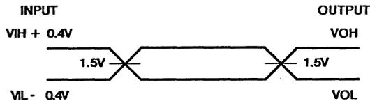
NOTE: Input test signals must switch between  $V_{IL}$  (maximum)  $-0.4\text{V}$  and  $V_{IH}$  (minimum)  $+0.4\text{V}$ .  $\overline{\text{RES}}$  and  $\overline{\text{F/C}}$  must switch between  $0.4\text{V}$  and  $V_{CC} - 0.4\text{V}$ . Input rise and fall times driven at  $1\text{ns/V}$ .  $V_{IL} \leq V_{IL}(\text{max}) - 0.4\text{V}$  for CSYNC pin.  $V_{CC} - 4.5\text{V}$  and  $5.5\text{V}$ .
