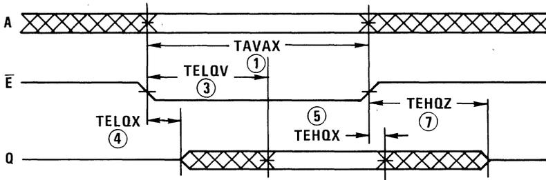
NOTE:  $\bar{W}$  is held high for entire cycle and D is ignored. Address is stable by the time  $\bar{E}$  goes low and remains valid until  $\bar{E}$  goes high.
