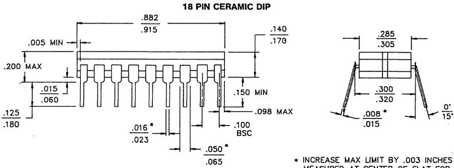
\* INCREASE MAX LIMIT BY .003 INCHES MEASURED AT CENTER OF FLAT FOR SOLDER FINISH
