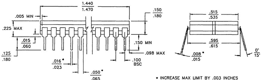
• INCREASE MAX LIMIT BY .003 INCHES MEASURED AT CENTER OF FLAT FOR SOLDER FINISH
