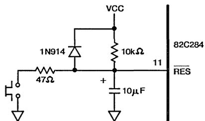
FIGURE 3. TYPICAL RC  $\overline{RES}$  TIMING CIRCUIT
