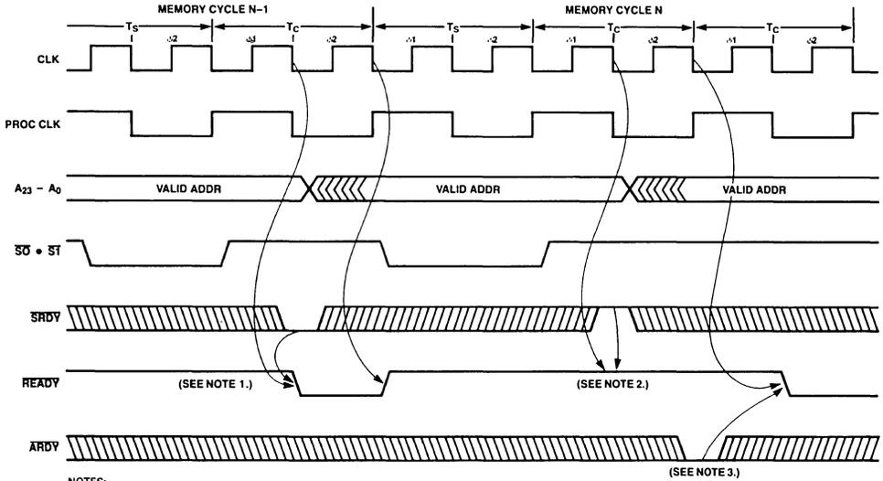
**FIGURE 25. SYNCHRONOUS AND ASYNCHRONOUS READY**
