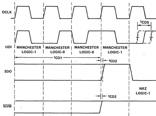
NOTE: Manchester Data In is not synchronous with Decoder Clock.
