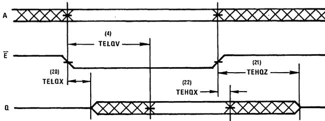
NOTE:  $\bar{W}$  is high for entire cycle and D is ignored. Address is stable by the time  $\bar{E}$  goes low and remains valid until  $\bar{E}$  goes high.
