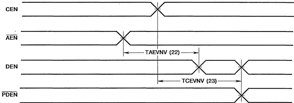
ADDRESS ENABLE ( $\overline{\text{AEN}}$ ) TIMING (THREE-STATE ENABLE/DISABLE)
