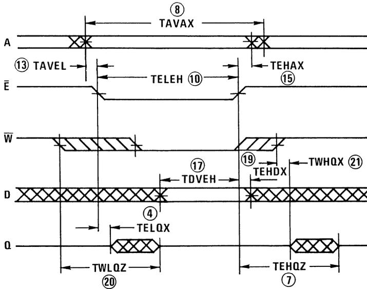
NOTE: In this mode,  $\bar{W}$  rises after  $\bar{E}$ . If  $\bar{W}$  falls before  $\bar{E}$  by a time exceeding  $TWLQZ$  (Max) -  $TELQX$  (Min), and rises after  $\bar{E}$  by a time exceeding  $TEHQZ$  (Max) -  $TWHQZ$  (Min), then Q will remain in the high impedance state throughout the cycle. The address must remain stable whenever  $\bar{E}$  and  $\bar{W}$  are both low.
