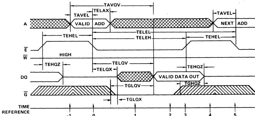
The address information is latched in the on chip registers on the falling edge of  $\bar{E}$  ( $T = 0$ ), minimum address setup and hold time requirements must be met. After the required hold time, the addresses may change state without affecting device operation. During time ( $T = 1$ ), the outputs become enabled but data is not valid until time ( $T = 2$ ),  $\bar{W}$  must re-
