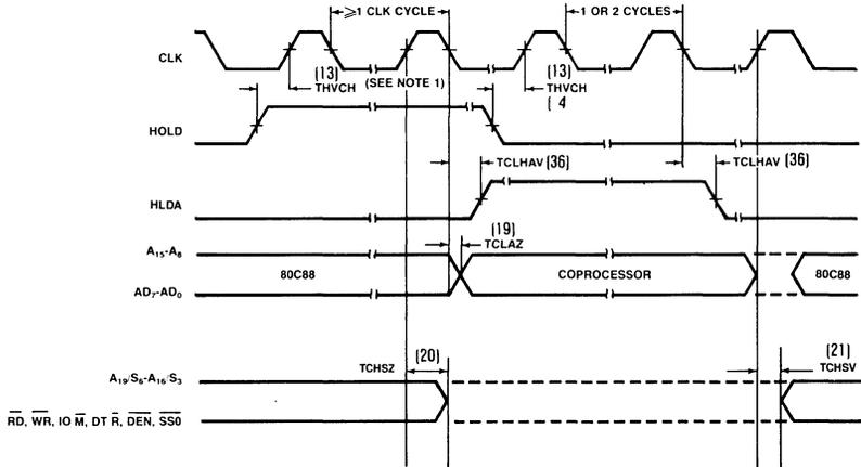
NOTE: Setup requirements for asynchronous signals only to guarantee recognition at next CLK
