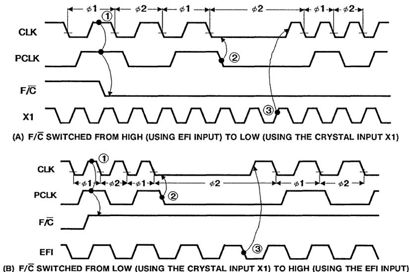
FIGURE 1. DYNAMICALLY SWITCHING THE  $F/\bar{C}$  PIN
