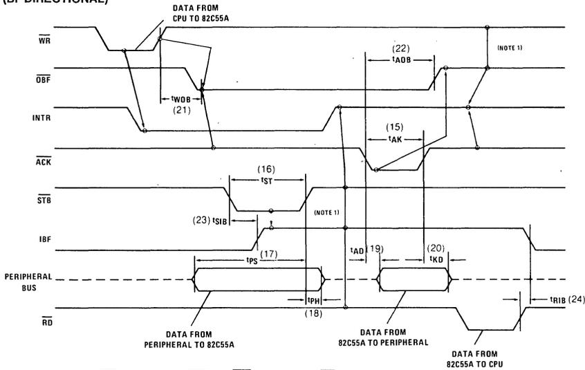
NOTE: 1. Any sequence where  $\overline{WR}$  occurs before  $\overline{ACK}$  and  $\overline{STB}$  occurs before  $\overline{RD}$  is permissible.
