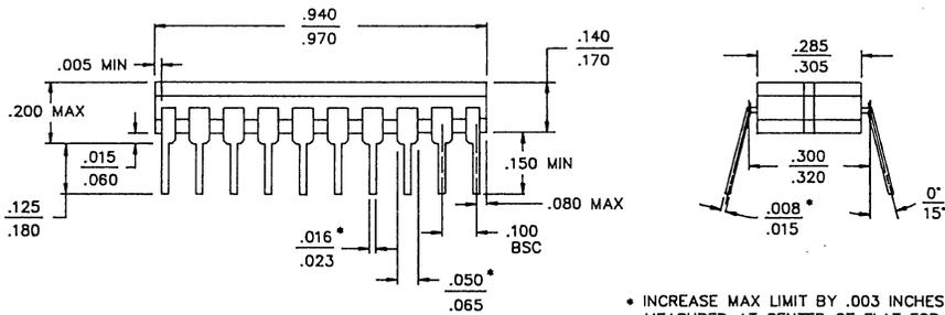
**LEAD MATERIAL:** Type B**LEAD FINISH:** Type A**PACKAGE MATERIAL:** Ceramic 90% Alumina**PACKAGE SEAL:**
