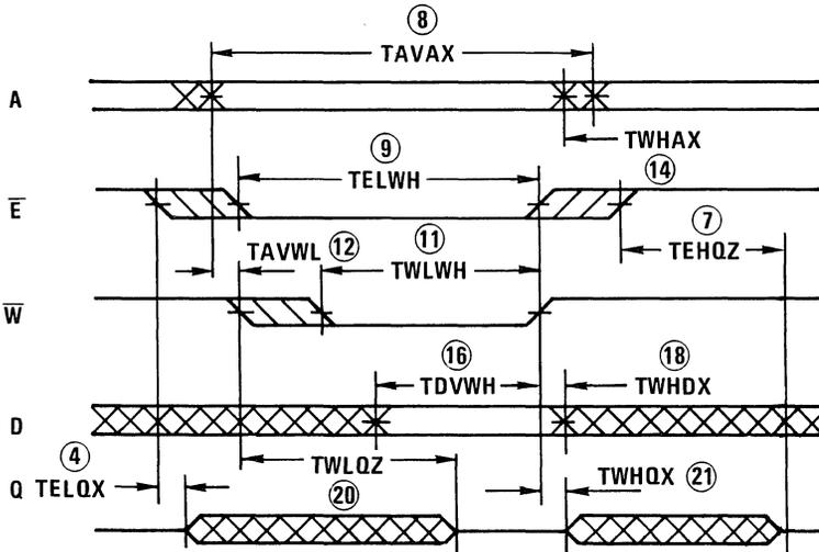
NOTE: In this mode,  $\bar{E}$  rises after  $\bar{W}$ . The address must remain stable whenever both  $\bar{E}$  and  $\bar{W}$  are Low.
