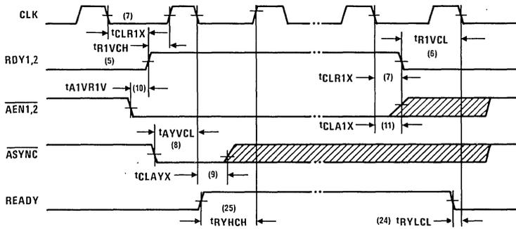
WAVEFORMS FOR READY SIGNALS (FOR SYNCHRONOUS DEVICES)
