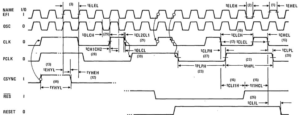
NOTE: All timing measurements are made at 1.5 Volts, unless otherwise noted.
