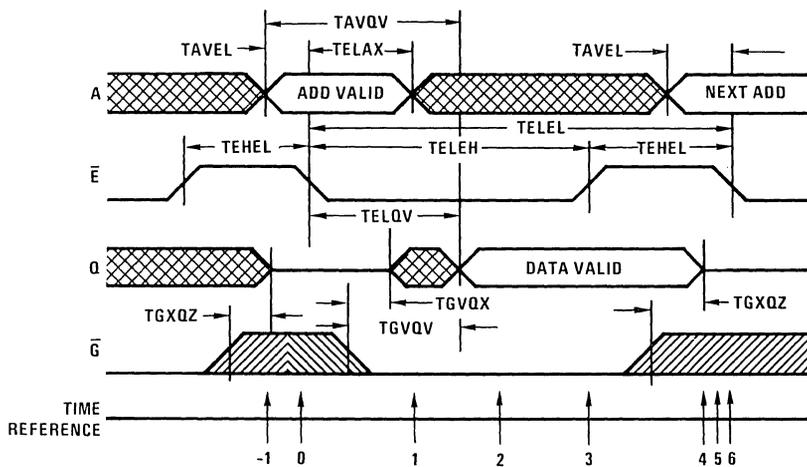
\* G Has the same timing as  $\bar{G}$  except signal is inverted.
