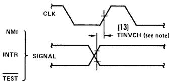
NOTE: Setup requirements for asynchronous signals only to guarantee recognition at next CLK
