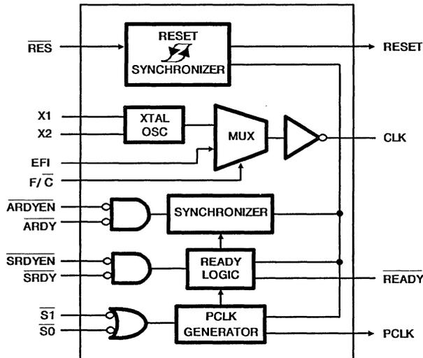
**Pin Description** The following pin function descriptions are for the 82C284/883 clock generator.
