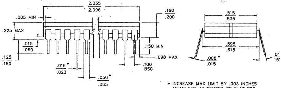
\* INCREASE MAX LIMIT BY .003 INCHES MEASURED AT CENTER OF FLAT FOR SOLDER FINISH
