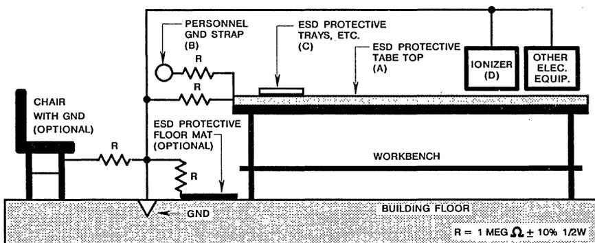
FIGURE 4. STATIC-SAFEGUARDED WORK STATION
