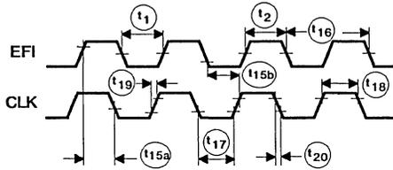
NOTE: The EFI input LOW and HIGH times as shown are required to guarantee the CLK LOW and HIGH times shown.
