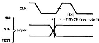
NOTE: Setup requirements for asynchronous signals only to guarantee recognition at next CLK
