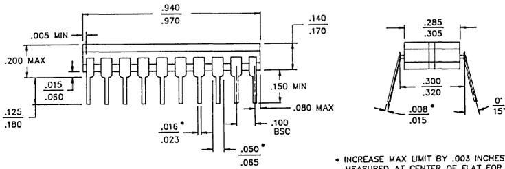
\* INCREASE MAX LIMIT BY .003 INCHES MEASURED AT CENTER OF FLAT FOR SOLDER FINISH
