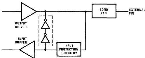
FIGURE 20A. BUS HOLD CIRCUITRY — PINS 36-51, 66, 67
