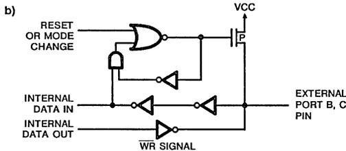
FIGURE 2. PORT A & B, PORT C BUS-HOLD CONFIGURATION
