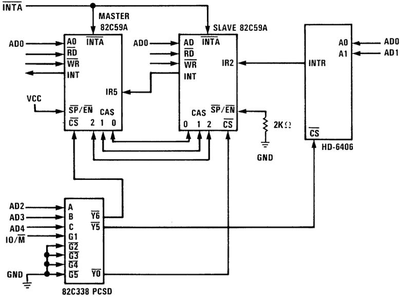
FIGURE 15. EXAMPLE 2: CASCADED 82C59As
