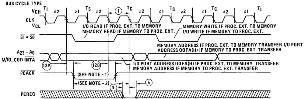
ASSUMING WORD-ALIGNED MEMORY OPERAND. IF ODD ALIGNED, 80C286/883 TRANSFERS TO/FROM MEMORY BYTE-AT-A-TIME WITH TWO MEMORY CYCLES.
