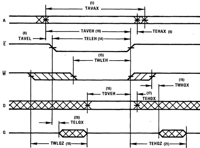
NOTE: In this mode,  $\bar{W}$  rises after  $\bar{E}$ . If  $\bar{W}$  falls before  $\bar{E}$  by a time exceeding  $TWLQZ$  (Max)  $TELOX$  (Min), and rises after  $\bar{E}$  by a time exceeding  $TEHQZ$  (Max)  $-TWHQZ$  (Min), then  $Q$  will remain in the high impedance state throughout the cycle.
