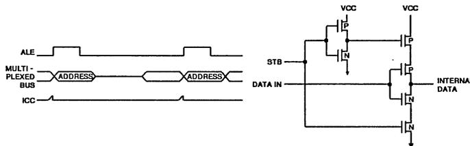
FIGURE 3. SYSTEM EFFECTS OF GATED INPUTS
