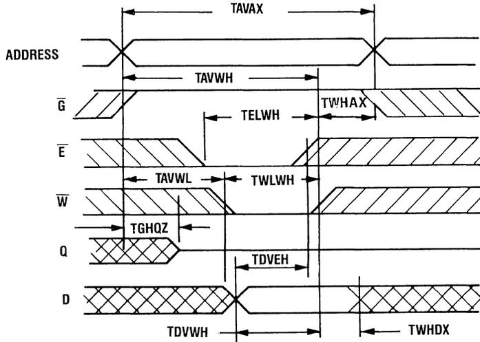
In this write cycle  $\bar{G}$  has control of the output after a period, TGHQZ.  $\bar{G}$  switching the output to a high impedance state allows data in to be applied without bus contention after
