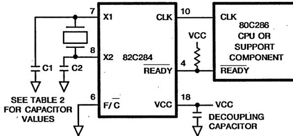
FIGURE 4. RECOMMENDED CRYSTAL AND READY CONDITIONS
