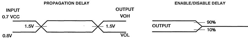
AC Testing: All input signals (except IX and RST) must switch between 0.8V and 0.7 VCC. Input rise and fall times are driven at 1nsec per volt.
