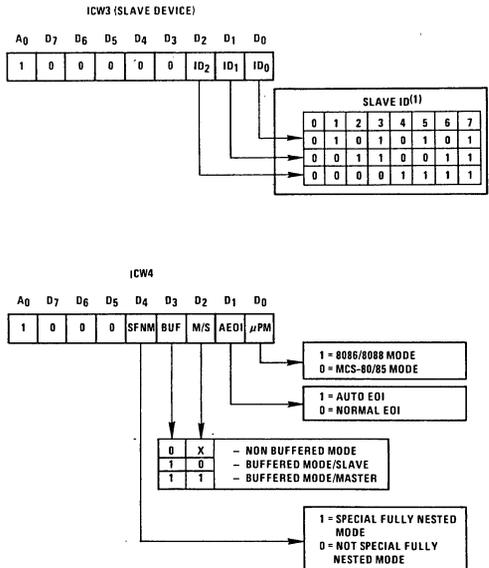
NOTE: Slave ID is equal to the corresponding master IR input
