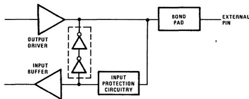
FIGURE 6A. BUS HOLD CIRCUITRY PIN 2-16, 35-39
