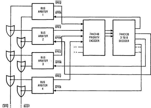
FIGURE 1. PARALLEL PRIORITY RESOLVING TECHNIQUE
