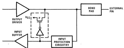
FIGURE 20B. BUS HOLD CIRCUITRY — PINS 4-6, 68
