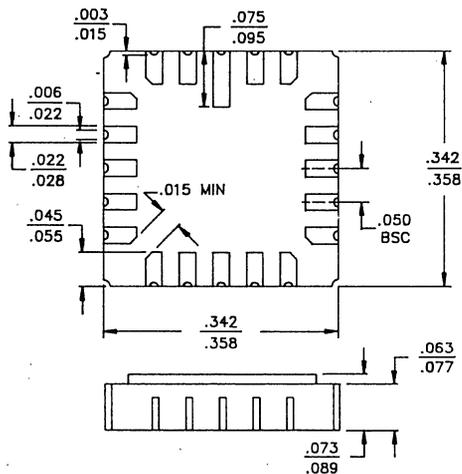
**PAD MATERIAL:** Type C**PAD FINISH:** Type A**FINISH DIMENSION:** Type A**PACKAGE MATERIAL:** Multilayer Ceramic, 90% Alumina**PACKAGE SEAL:**
