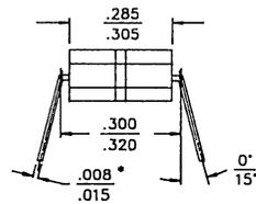
\* INCREASE MAX LIMIT BY .003 INCHES MEASURED AT CENTER OF FLAT FOR SOLDER FINISH
