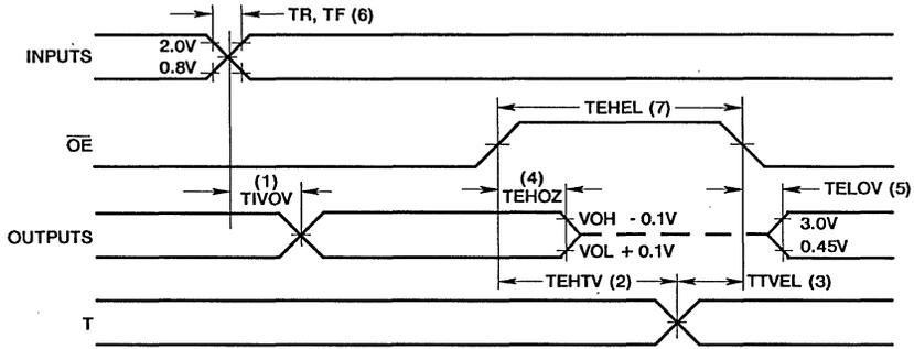
All timing measurements are made at 1.5V unless otherwise noted
