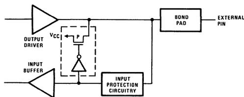
FIGURE 6B. BUS HOLD CIRCUITRY PIN 26-32, 34
