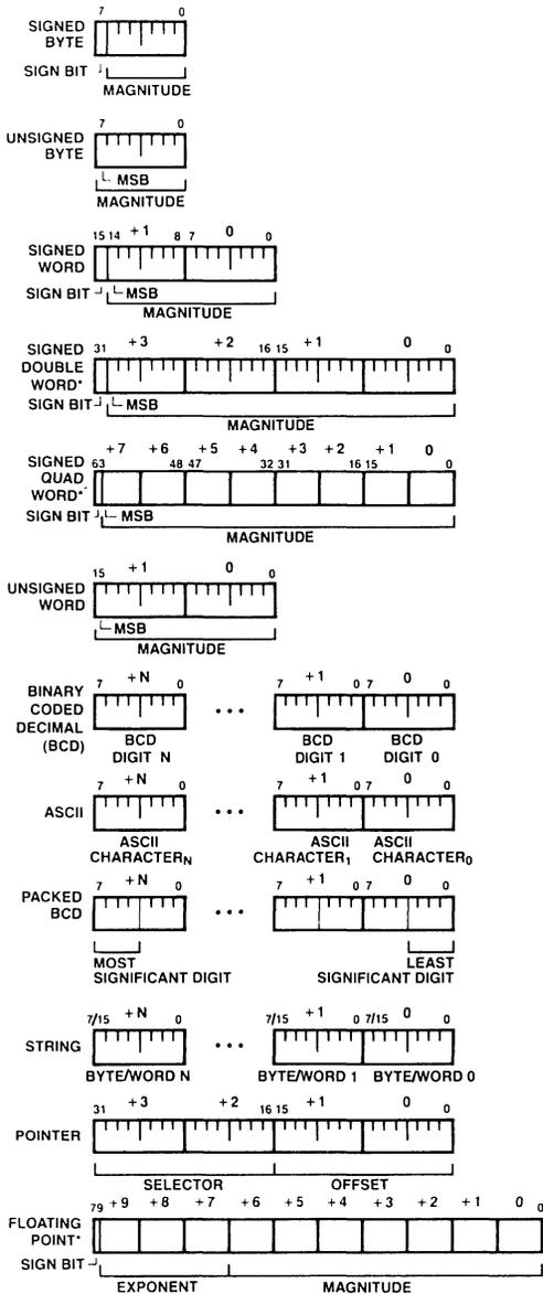
\*Supported by 80C286 80287 Numeric Data Processor Configuration
