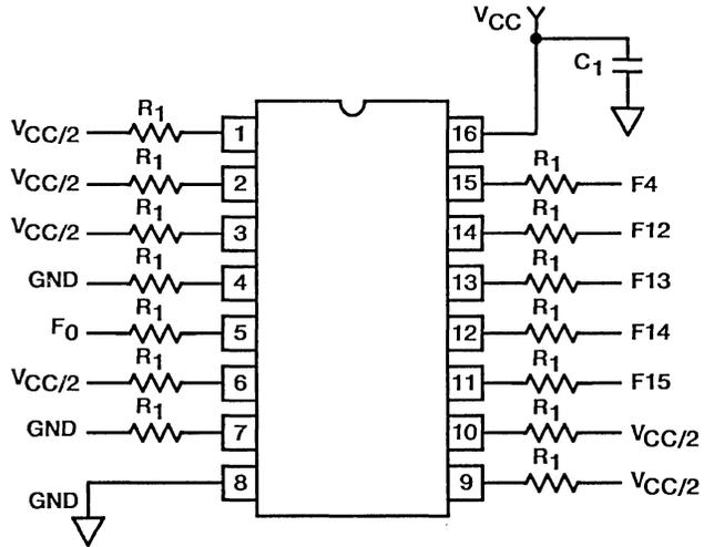
NOTES:  $F_0 = 100\text{KHz} \pm 10\%$ ,  $F_1 = F_0/2$ ,  $F_2 = F_1/2, \dots$
