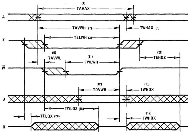
NOTE: In this mode,  $\bar{E}$  rises after  $\bar{W}$ . The address must remain stable whenever both  $\bar{E}$  and  $\bar{W}$  are low.
