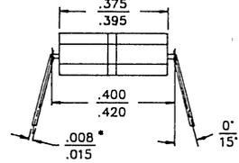
\* INCREASE MAX LIMIT BY .003 INCHES MEASURED AT CENTER OF FLAT FOR SOLDER FINISH
