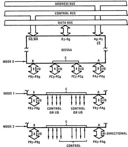
FIGURE 3. BASIC MODE DEFINITIONS AND BUS INTERFACE
