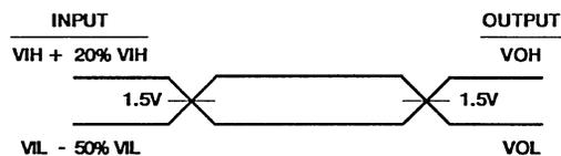
A.C. Testing: All input signals (other than CLK) must switch between  $V_{ILmax} - 50\% V_{IL}$  and  $V_{IHmin} + 20\% V_{IH}$ . CLK must switch between 0.4V and  $V_{CC} - 0.4V$ . Input rise and fall times are driven at 1ns/V.
