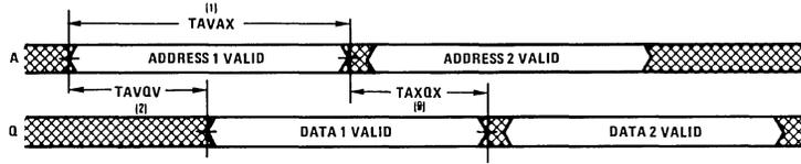
READ CYCLE 2: E, S, or  $\overline{G}$  CONTROLLED (NOTE 1)
