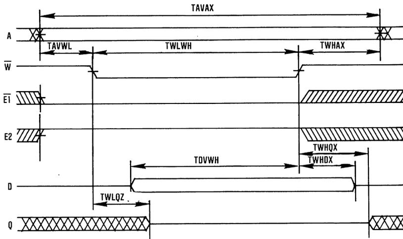
WRITE CYCLE II: EARLY WRITE - CONTROLLED BY  $\bar{E1}$
