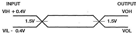
A.C. Testing: All input signals (other than CLK) must switch between  $V_{IL}-0.4V$  and  $V_{IH}+0.4V$ . CLK must switch between  $0.4V$  and  $V_{CC}-0.4V$ . Input rise and fall times are driven at 1ns/V.
