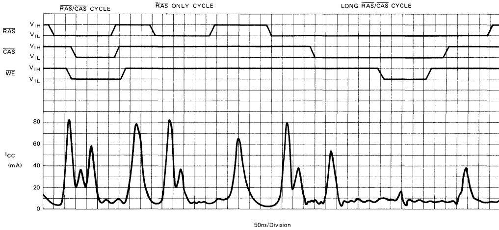
FIG. 2 — CURRENT WAVEFORMS ( V_{CC} = 5.0V, T_A = 25^\circ C )
