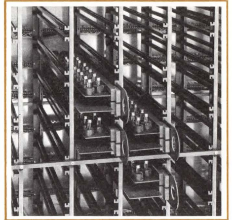
Life testing equipment for high reliability devices such as those used in telemetry systems in NASA's Interplanetary Platform (IMP) satellites. Mounting boards are designed to permit device operation and testing at 125°C.
