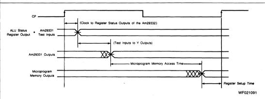
Figure 9. Cycle Timing Waveform\*
