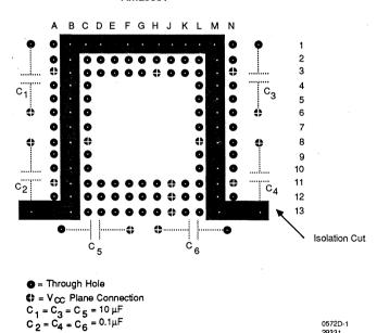
Figure 7-1a. Layout Recommendations for the  $\rm V_{cc}\,$  Plane
