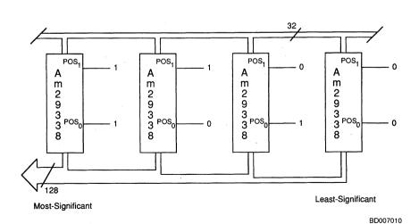
Figure 3. Position Line Values in Horizontally Cascaded System
