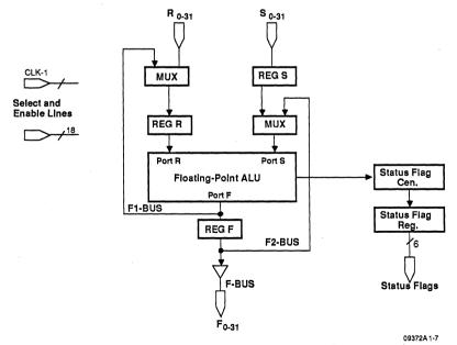
Figure 1-7. Am29325/29C325 32-Bit Floating Point Processor
