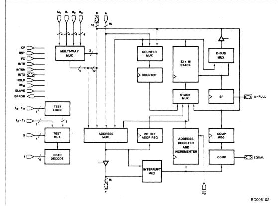
Figure 1. Am29C331 Detailed Block Diagram
