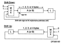
Figure 5. Upshift/Downshift Using Link Bit
