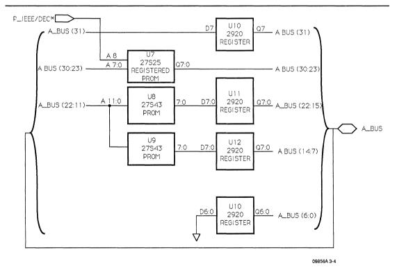
Figure 3-4. Floating Point Block Seed Look-Up Table -- Data Flow Diagram
