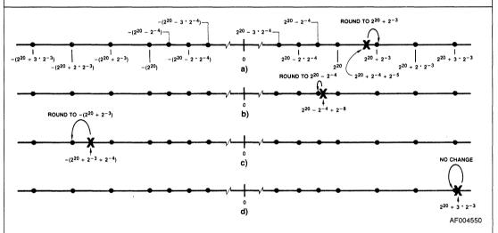
Figure 9. Floating-Point Rounding Examples for Round-to-Nearest Mode
