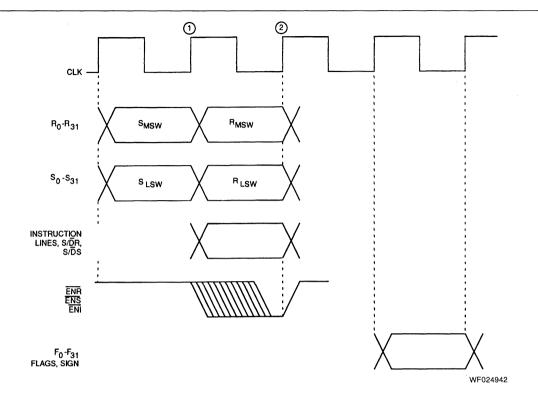
Timing of Operations with Input Mode 8 (64-Bit Bus, Double-Cycle, S First)\*
