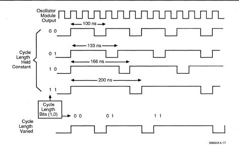
Figure 5-17. Clock Generator Outputs (Inverted)
