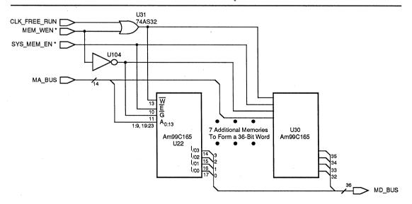
The memory address counters are loadable up/down counters that can serve as address pipeline registers, sequencers, or stack pointers independent of the CPU's data section. They allow sequential reads or writes to memory by the CPU without requiring the CPU to calculate an address on every read or write cycle.
