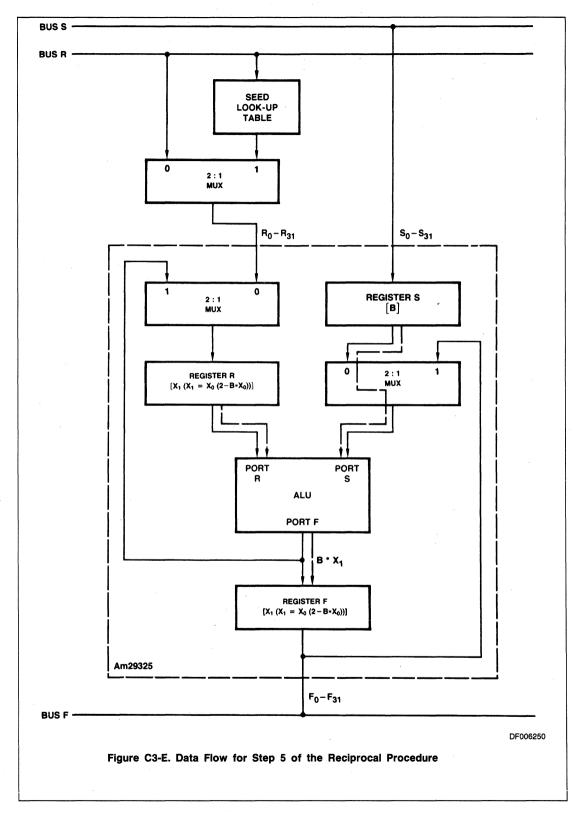
A tabular description of the operations above is given in Table C3. The following examples, performed in IEEE format. illustrate the process.
