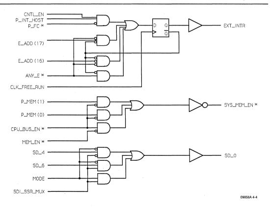
Figure 4-4. U17 Am22V10A Host Interface Glue Logic
