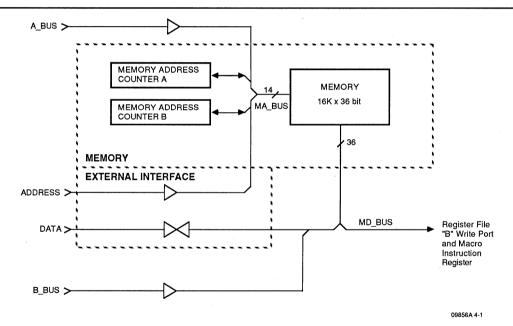
Figure 4-1. Memory and External Interface Address and Data Paths
