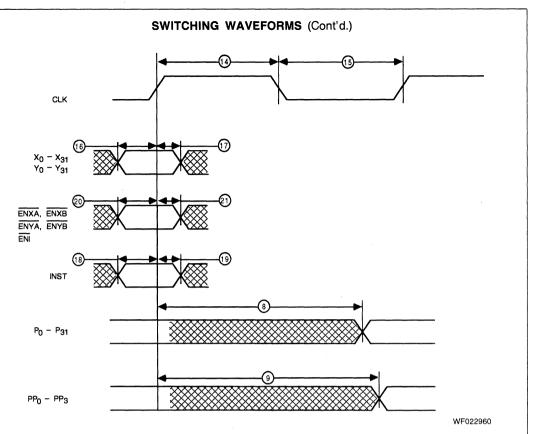
Clocked Operation: Output Taken from Adder (FTX, Y, I = LOW; FTP = HIGH; PSEL1  $\neq$  PSEL0)
