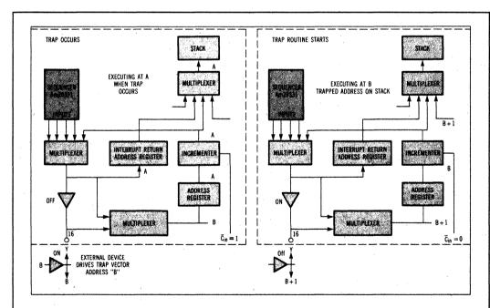
Errors are signaled with Parity-Error and MS-Error outputs and prioritized by an interrupt controller. The sequencers then trap the microinstruction that is being executed. To restart a microinstruction when a failure occurs, the sequencer can perform traps at any microinstruction boundary. When a trap condition is signaled, the sequencer changes the Y output bus to a high-impedance state, allowing an external trap to be placed on it.
