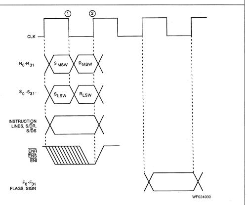
Timing of Operations with Input Mode 6 (64-Bit Bus, Single-Cycle, S First)\*
