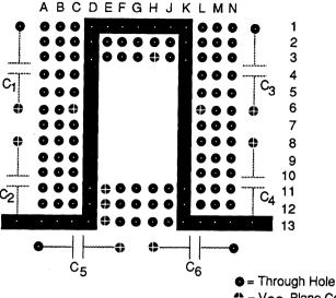
$\Leftrightarrow$  = V<sub>CC</sub> Plane Connection C<sub>1</sub> = C<sub>3</sub> = C<sub>5</sub> = 10  $\mu$ F or greater (electrolytic
