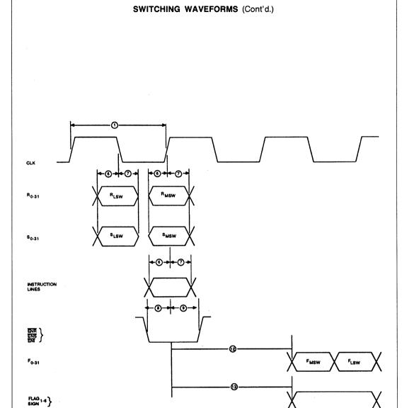
Timing of Operations with F-Register and Status Register in Feedthrough Mode. Assumes 32-Bit Bus, Single-Cycle, LSW-First Input Mode and Flow-Through Operation.
