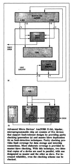
parity-generation system. Byte-write capability provides other advantages. In byte parity, individual bytes can be written back into the register file without reading the rest of the 32-bit word to compute parity.
