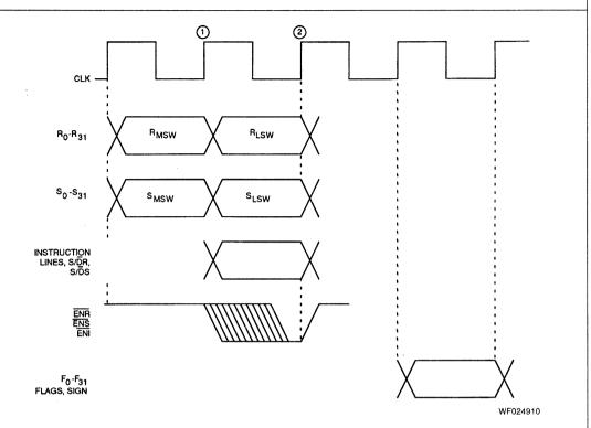
Timing of Operations with Input Mode 4 (32-Bit Bus, Double-Cycle, MSW First)\*
