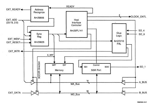
Figure 4-2. Host Interface Block Diagram
