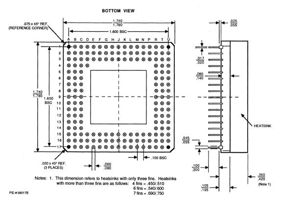
NOTE: Package dimensions are given in inches. To convert to millimeters, multiply by 25.4.
