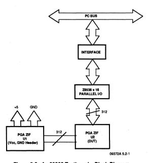
Figure 5-3. Am29300 Testboard - Block Diagram
