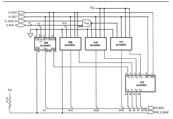
Figure 5-10. D Bus Transceiver
