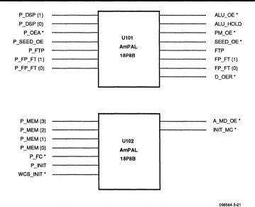
Figure 5-21. Control Decode Logic Part1
