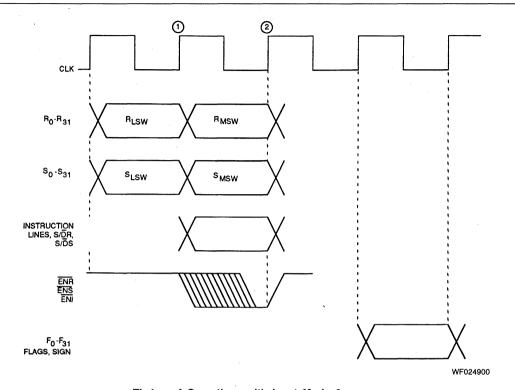
Timing of Operations with Input Mode 3 (32-Bit Bus, Double-Cycle, LSW First)\*
