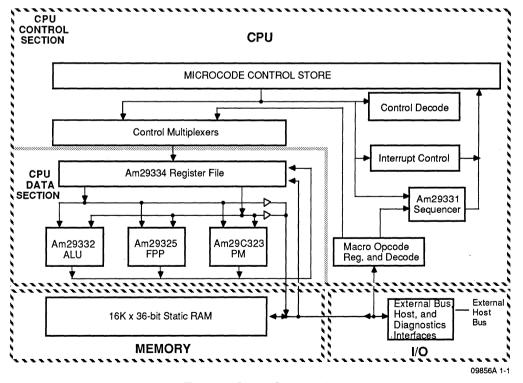
Figure 1-1. System Components
