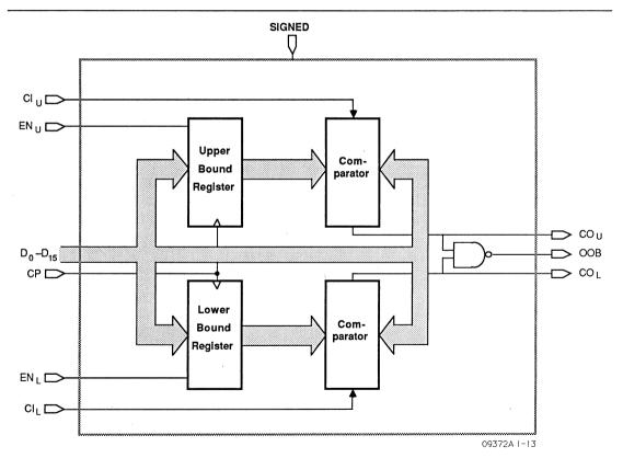
Figure 1-13. Am29337 Block Diagram
