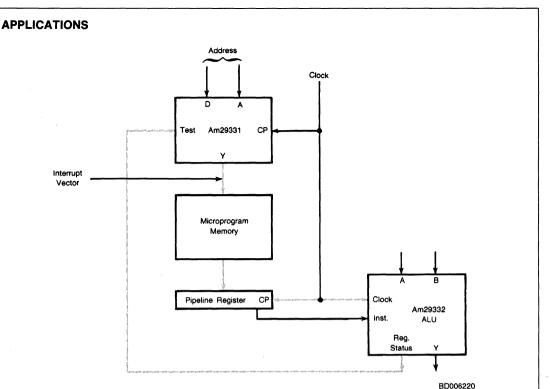
Figure 8. Typical Control-Path Architecture For Am29300 Family
