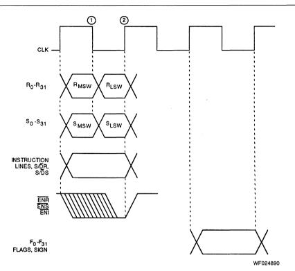
Timing of Operations with Input Mode 2 (32-Bit Bus, Single-Cycle, MSW First)\*
