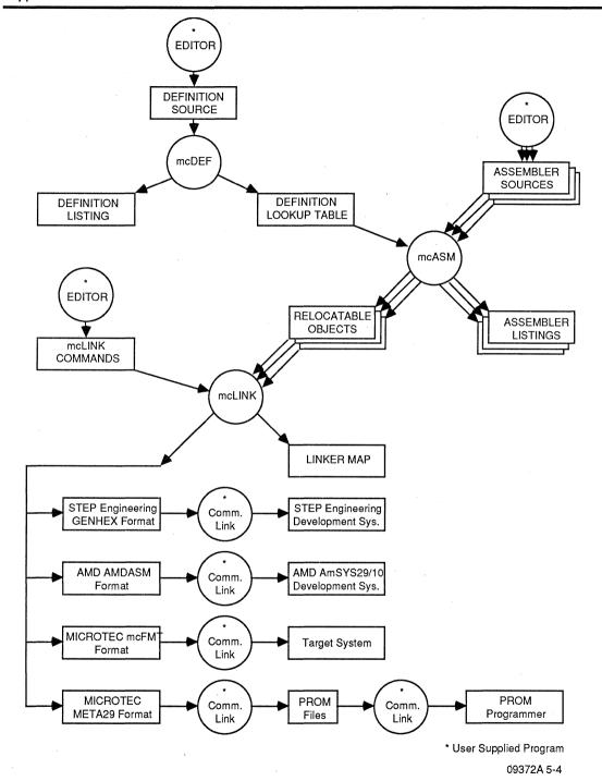
Figure 5-4. Overview of the Microtec Research mcASM Development Process
