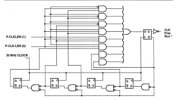
Figure 5-16. U100 AmPAL16R6B Clock Generator
