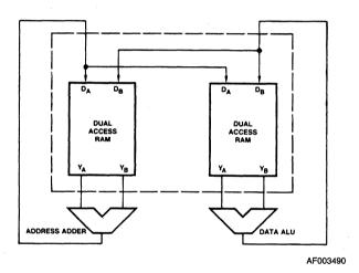
Figure 3. RAM with 4 Read Ports and 2 Write Ports
