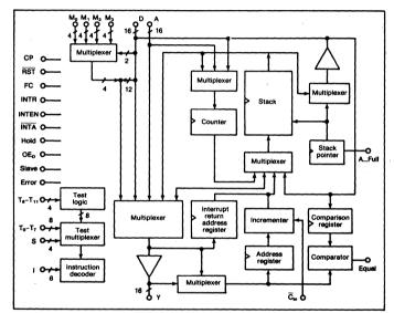
5. To aid in handling trap operations, the incrementer is placed after the address register in the Am29331 microsequencer. Additionally, the chip has a 16-bit address bus, which enables it to access up to 64 kwords of control memory and handle interrupts and multiple-path branches.
