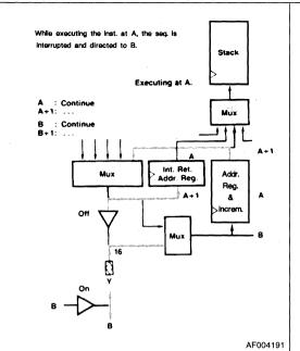
Figure 4. Am29C331 Interrupt Cycle 1
