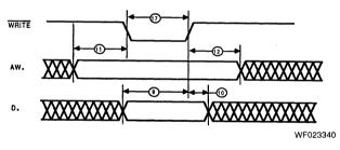
Write Function (\* means A or B)
