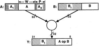
If position ( $P_0$ - $P_5$ ) < 0, B is LSB aligned Width ( $W_0$ - $W_5$ ) = 1 to 32
