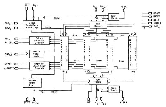
Figure 1. Am29338 Byte Queue Detailed Block Diagram
