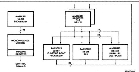
Figure 2. Am29C332 Family High-Performance System Block Diagram
