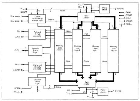
1. The Am29338 Byte Queue from AMD is a generalpurpose, 32-bif FIFO buffer with four 8-by-32-bif RAM memory stacks. It works in either the synchronous or synchronous mode, can transmit data blocks, and performs error checking at both input and output. Up to four bytes can be queued or dequeued in one cycle (a). Each stack has its own pointers: queue and dequeue logic enabling variable-width data to enter and leave the FIFO buffer (b).
