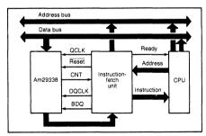
The FIFO buffer can function as an instruction-prefetch queue by coupling it with a separate instruction-fetch unit. The CPU runs faster by reading repetitive instruction loops from the byte queue without addressing main memory.
