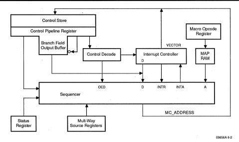
Figure 6-2. Control Section Timing Paths
