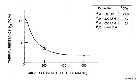
Figure 11. Am29331 Thermal Characteristics (Typical)
