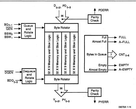
Figure 1-14. Am29338 Block Diagram
