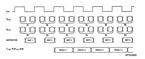
Figure 4. Timing for All Operations EXCEPT Multiply-Accumulate, Flow-Through Mode
