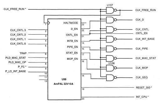
Figure 5-15. Clock Qualification Block Diagram
