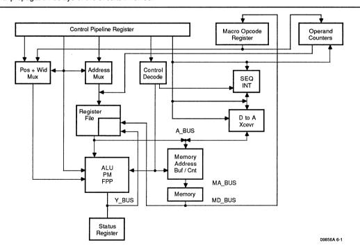
Figure 6-1. Data Section Timing Paths
