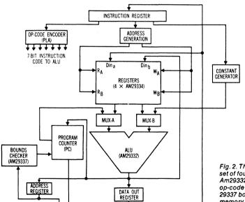
Fig. 2. The AMD RISC system includes a set of four Am29334 registers and an Am29332 ALU, which derives its 7-bit op-code controls from a PLA. The Am-29337 bounds checker identifies all memory references to the file registers.
