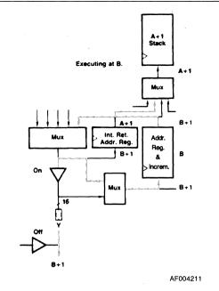
Figure 5. Am29C331 Interrupt Cycle 2
