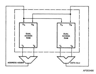
Figure 3. RAM with Four Read Ports and Two Write Ports
