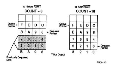
Figure 5. Retransmit Function with the Am29338
