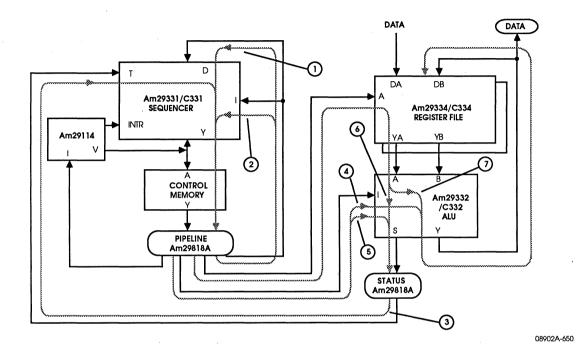
Figure 7-1. Am29300/29C300 System Timing Analysis
