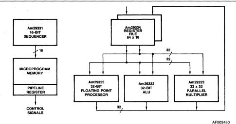
Figure 2. Am29332 Family High-Performance System Block Diagram
