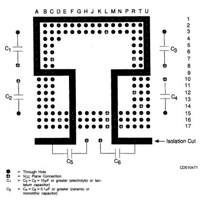
Figure 7. Suggested Printed Circuit-Board Layout
