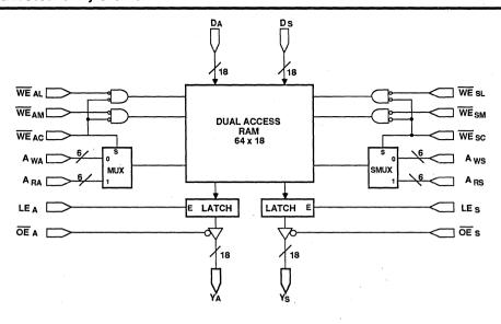
Figure 1-5. Am29334/29C334 Non-Pipelined Mode
