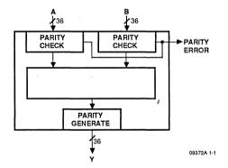
Figure 1-11. Input Parity Checking / Output Parity Checking
