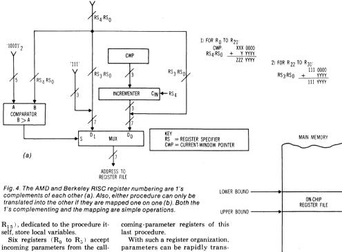
Six registers ( $\mathbf{R}_0$  to  $\mathbf{R}_5$ ) accept incoming parameters from the calling procedure for use by the called procedure. They are also used to return results from the called to the calling procedure.
