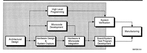
Figure 5-9. Microprogrammed Product Development Cycle (with simulating)
