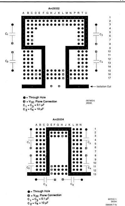
Figure 7-1b. Layout Recommendations for the  $\rm V_{cc}$  Plane
