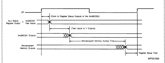
Figure 9. Cycle Timing Waveform\*
