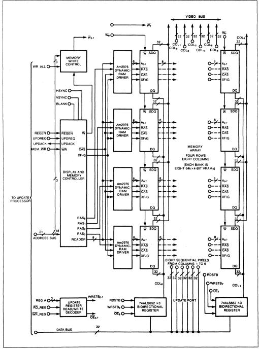
Fig 2—This frame buffer is organized as 2k pixels×1k lines×32 bits. Three-dimensional applications can read or write eight adjacent pixels at one time. For 2-D applications, each 32-bit word represents four 8-bit pixels.
