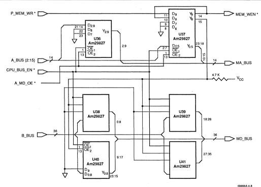
Figure 4-8. CPU to Memory Bus Buffers
