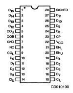
Note: Pin 1 is marked for orientation.
