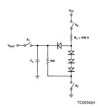
Notes: 1.  $C_L = 50 pF$  includes scope probe, wiring and stray capacitances without device in test fixture.
