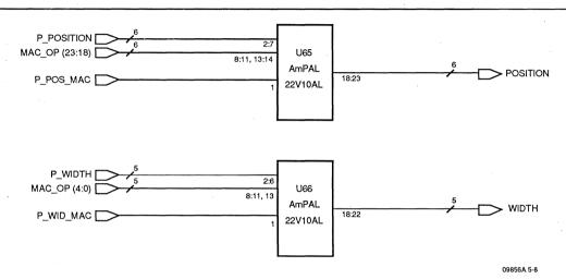
Figure 5-8. Position and Width MUX
