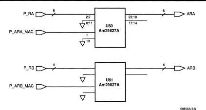
Figrue 5-5. Register File Address MUX, Read Ports
