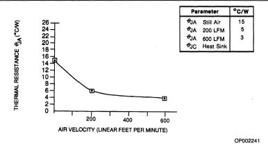
Figure 8. Am29332 Thermal Characteristics (Typical)
