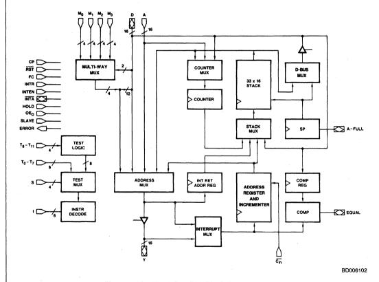
Figure 1. Am29331 Detailed Block Diagram
