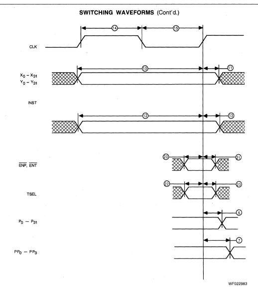
Clocked Operation: Input Registers Bypassed (FTX, Y, I = HIGH; FTP = LOW)
