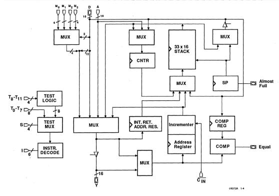
Figure 1-4. Am29331/29C331 16-Bit Microinterruptible Sequencer
