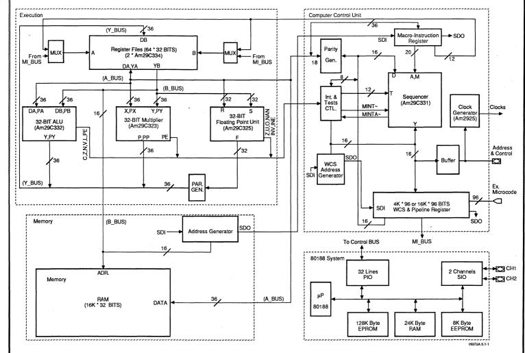
Figure 5-1. Am29C300 Evaluation Board
