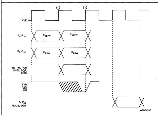
Timing of Operations with Input Mode 7 (64-Bit Bus, Double-Cycle, R First)\*
