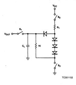
$$R_1 = \frac{5.0 - V_{BE} - V_{OL}}{I_{OL} + \frac{V_{OL}}{1K}}$$
