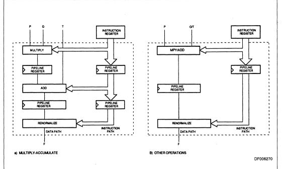
Figure 3. ALU Configuration for Double-Pipelined Mode
