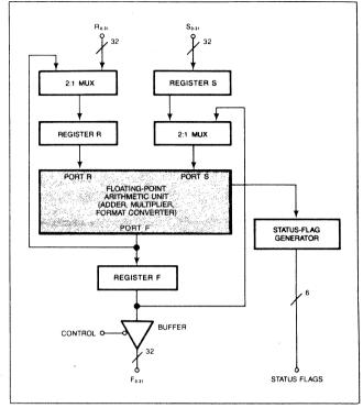
Fig A—This VLSI floating-point processor is fast because it contains all the major components for 32-bit operations on a single chip. It has one input for an external clock and 17 inputs for instruction-select and control functions.
