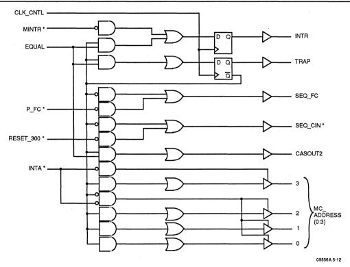
Figure 5-12. U75 AmPAL 22V10A Trap Logic PAL
