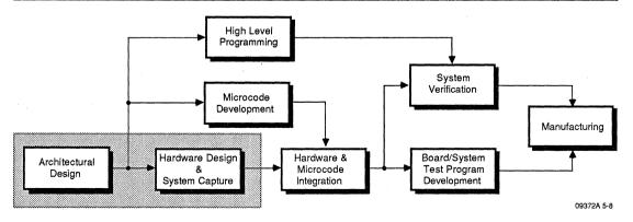
Figure 5-8. Microprogrammed Product Development Cycle (without simulating)
