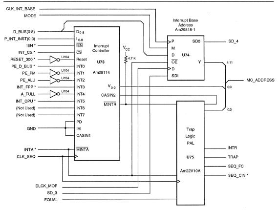
Figure 5-11. Interrupt and Trap Logic
