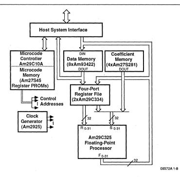
Figure 1-8. Microcoded Floating Point Co-Processor
