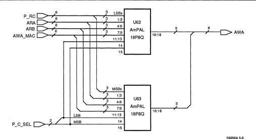
Figure 5-6. Register File Address MUX, Write Port A
