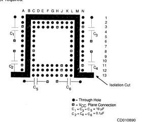
Figure 11. Suggested Printed Circuit-Board Layout
