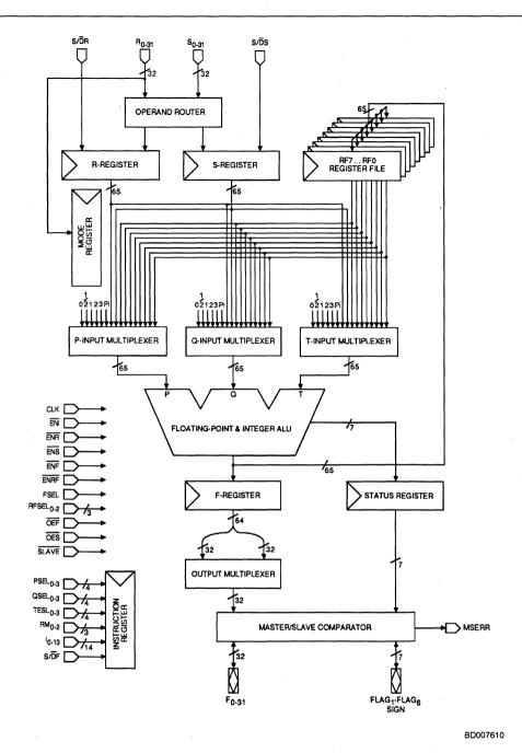
Figure 1. Am29C327 Double-Precision Floating-Point Processor
