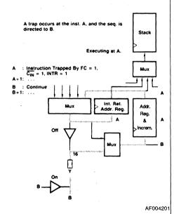
Figure 6. Am29C331 Traps Cycle 1
