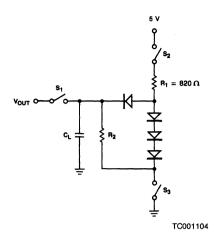
$$R_1 = I_{OL} + \frac{V_{OL}}{1K}$$
