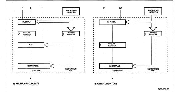
Figure 2. ALU Configuration for Single-Pipelined Mode
