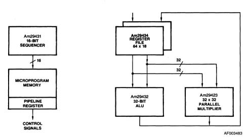
Figure 1. Am29400 Family High-Performance System Block Diagram
