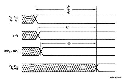
Flow-Through Operation (FT<sub>0</sub> = HIGH, FT<sub>1</sub> = HIGH)
